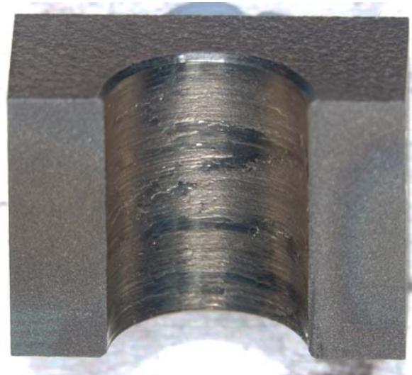
Figure 11. Surface photographs of smeared hole material – Type 6 anomaly.
