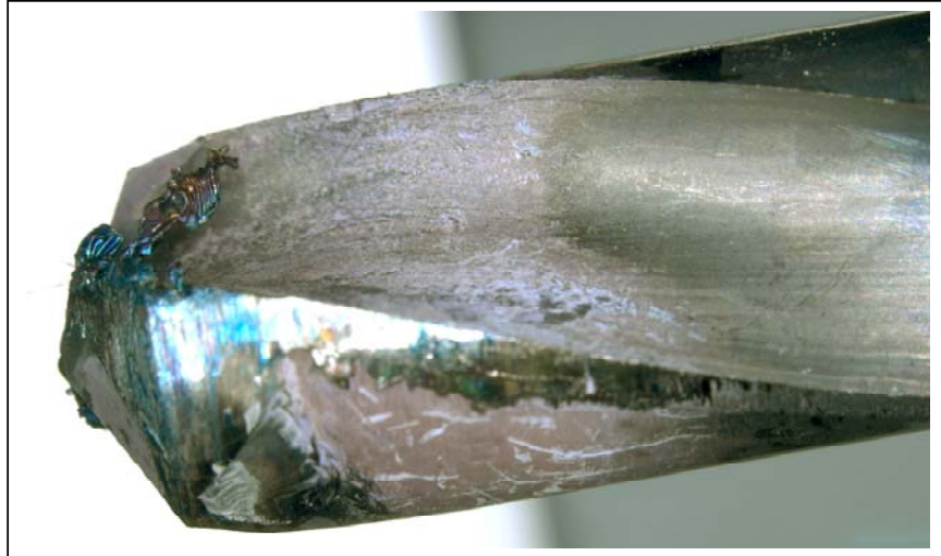
Figure 10. Example of a tool with significant adhered material. This tool was used to fabricate Type 6 anomalies in In718.
