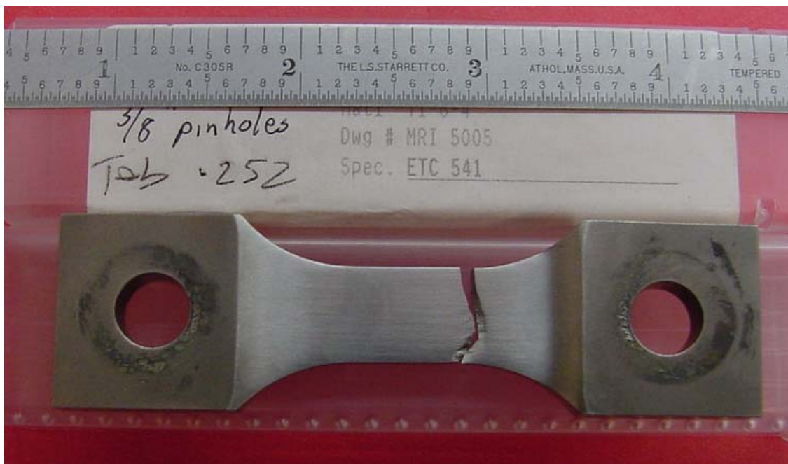
Figure 4. Pinned HCF specimen with edge radius transition failure.
