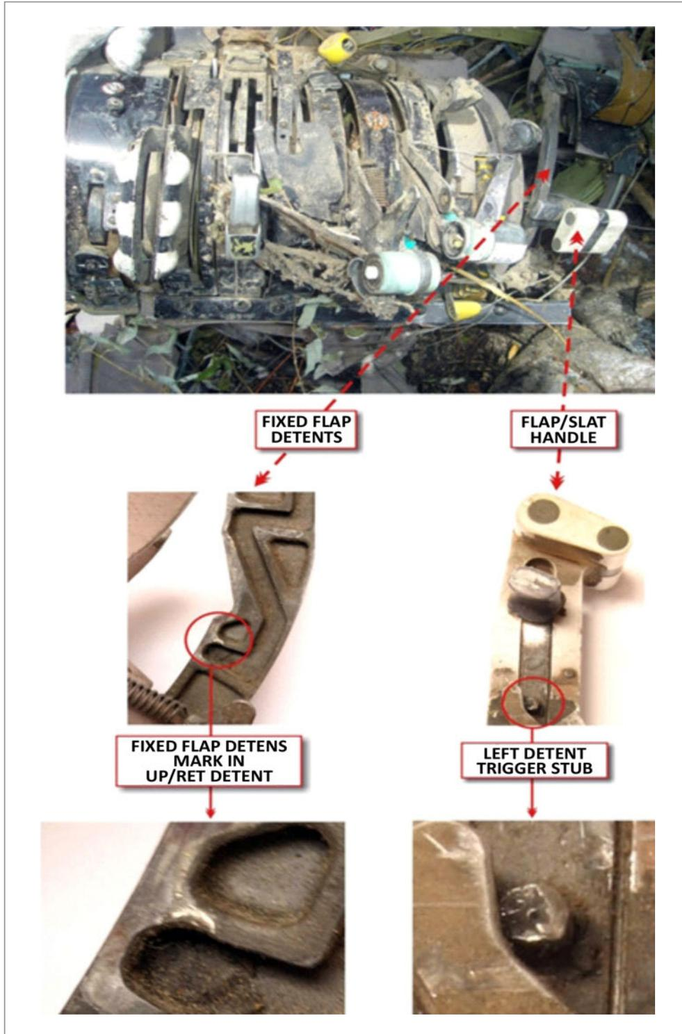
Figure 21. Close-ups of the flap/slat control lever
