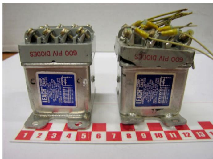
Figure 24. Comparison between the recovered relay and a new one of the same model
