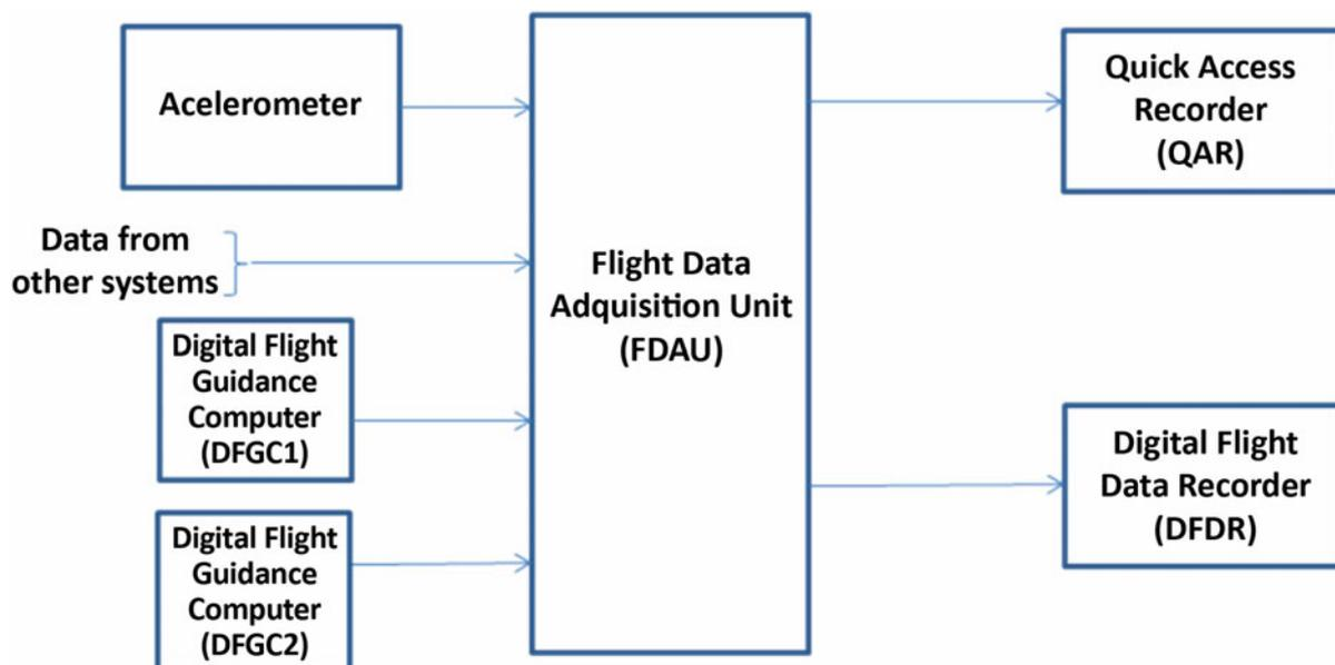
Figure 6. Architecture of flight data recording system
