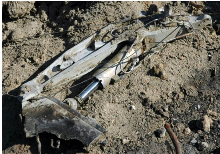
Figure 14. Part of outboard left flap and central actuator
