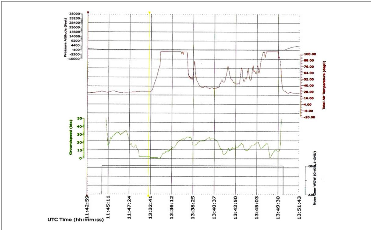
Figure 25. High RAT probe temperature events recorded on the DFDR (cont.)
