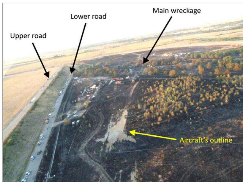
Figure 13. Aerial view of the path taken by the aircraft, showing the outline left by the aircraft on the ground
