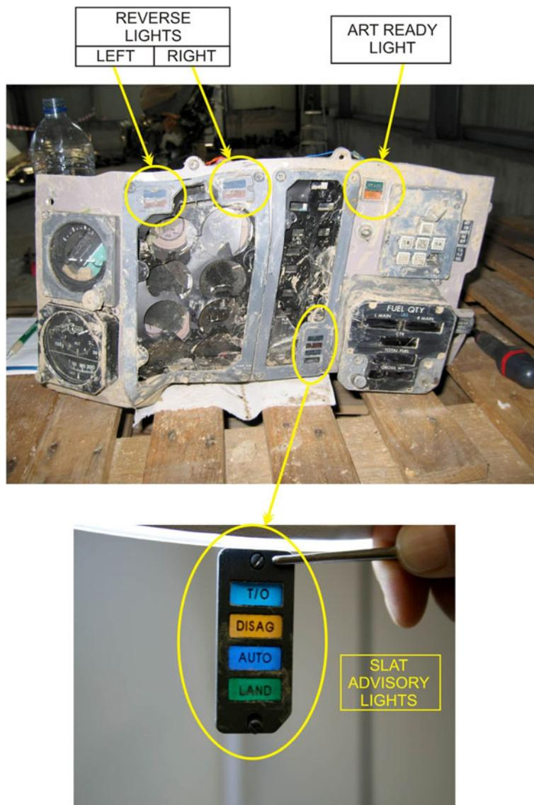
Figure 22. Center instrument panel
