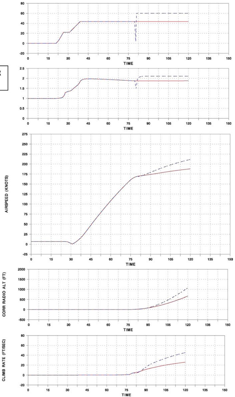
Figure 27. Effect of momentary power reduction to EPR of 1.65 and then increase to EPR of 2.20
