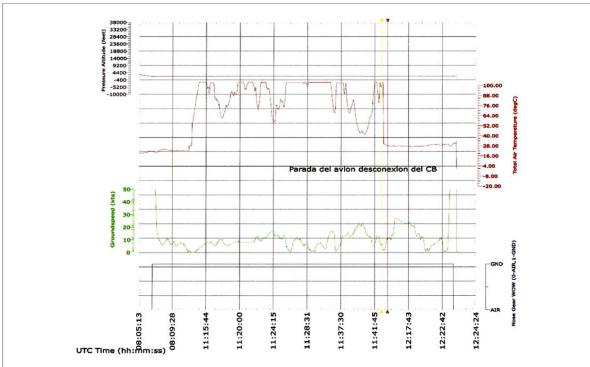
Figure 25. High RAT probe temperature events recorded on the DFDR (cont.)
