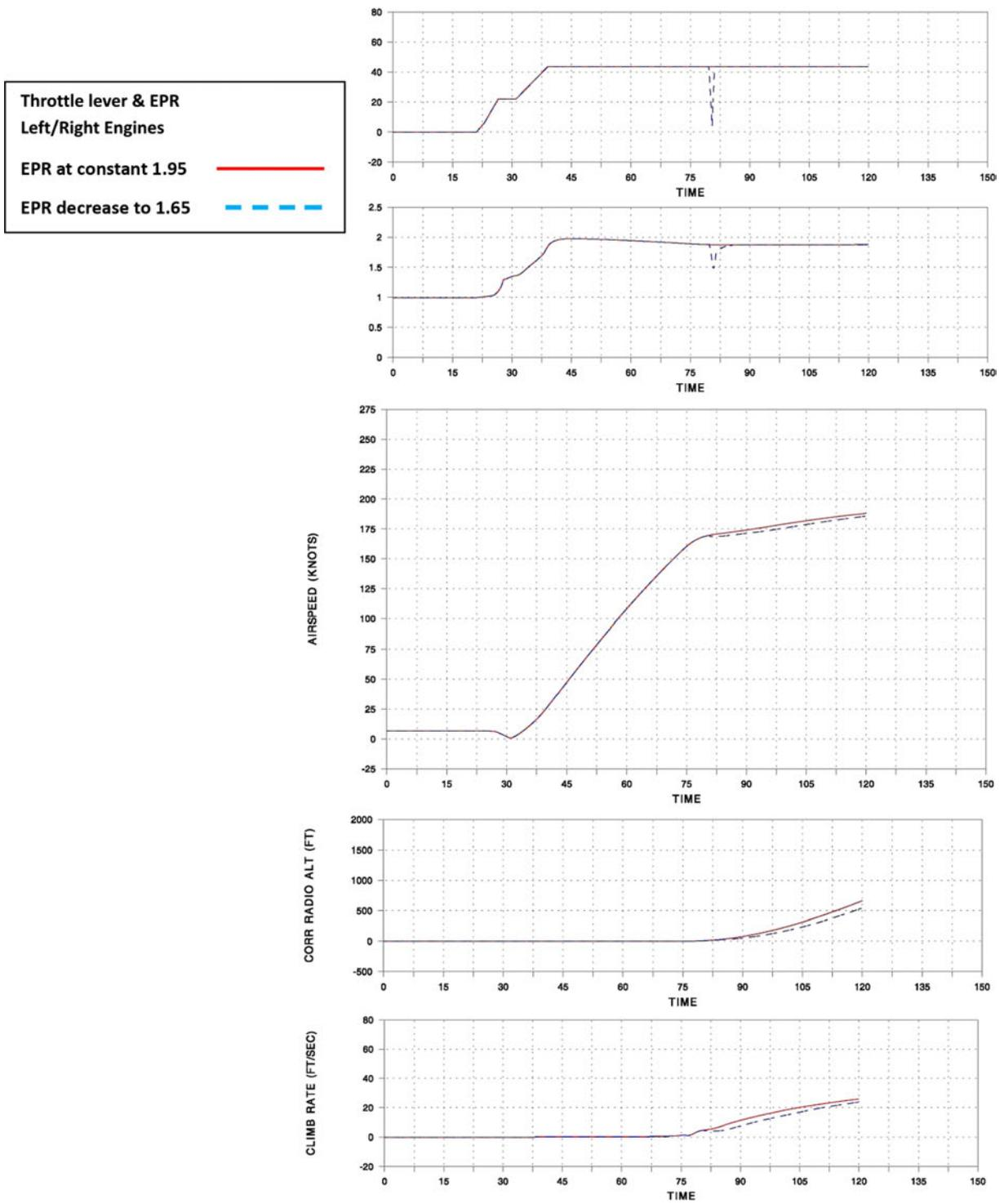
Figure 26. Effect of momentary reduction in EPR from a constant 1.95
