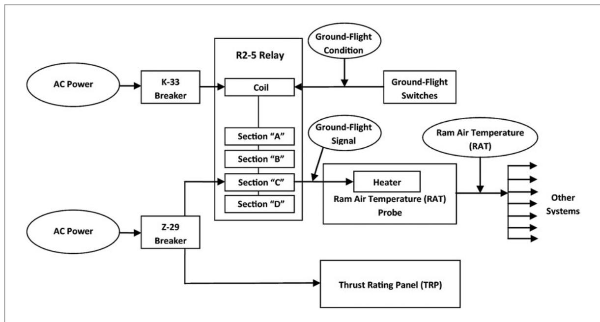
Figure 5. Diagram of RAT probe heater
