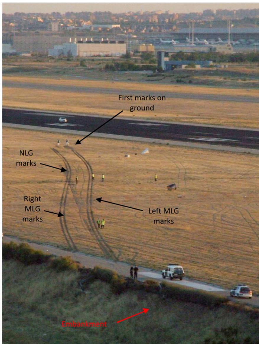
Figure 12. Tracks left by the aircraft as it traveled over the runway strip
