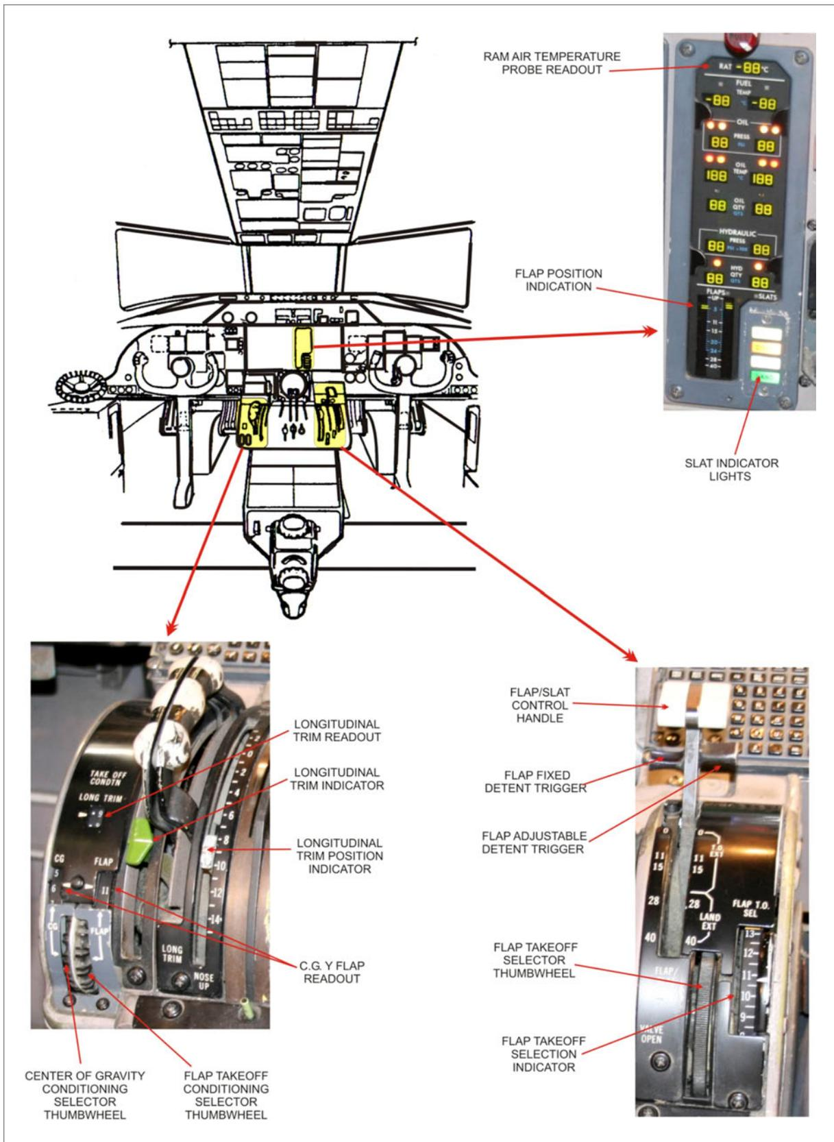
Figure 2. Flaps/slats controls and indicators
