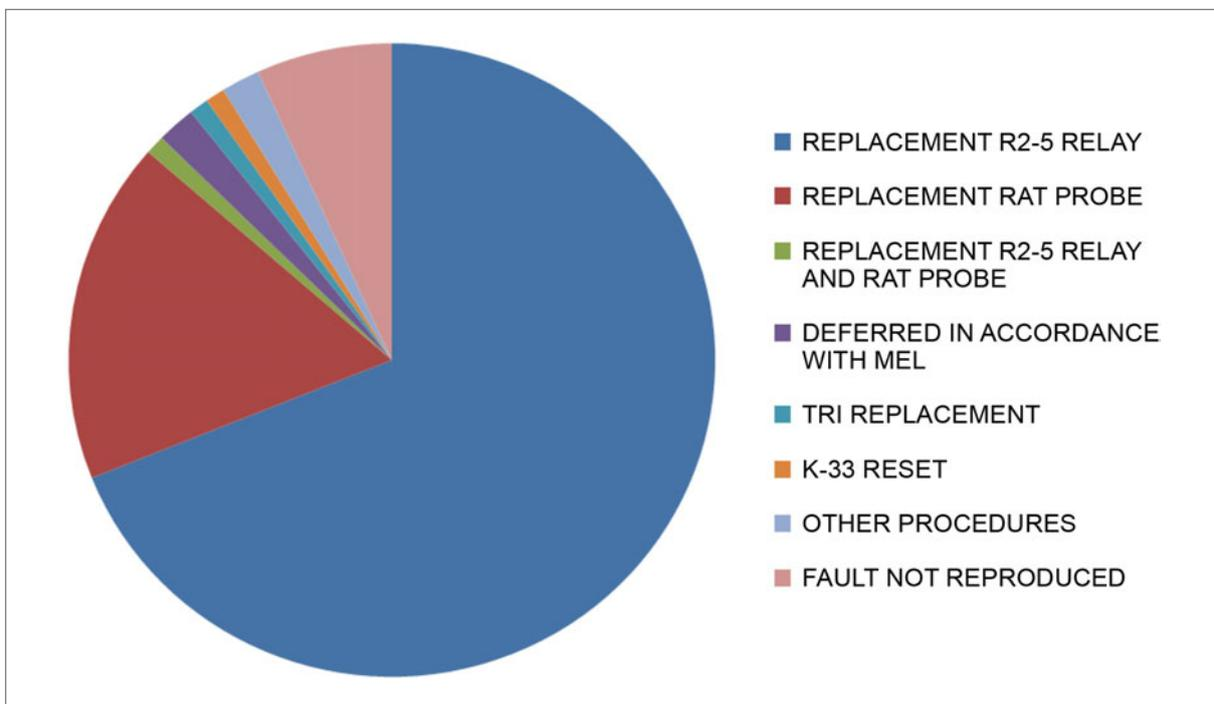
Figure 29. Previous high RAT probe temperatures on the ground. Cases compiled by Boeing (from 2000-2008)
