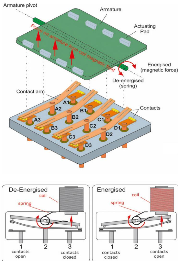
Figure 4. Interior of R2-5 relay
