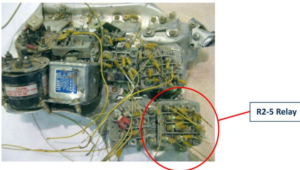
**Figure 23.** Recovered relay assembly housing R2-5
