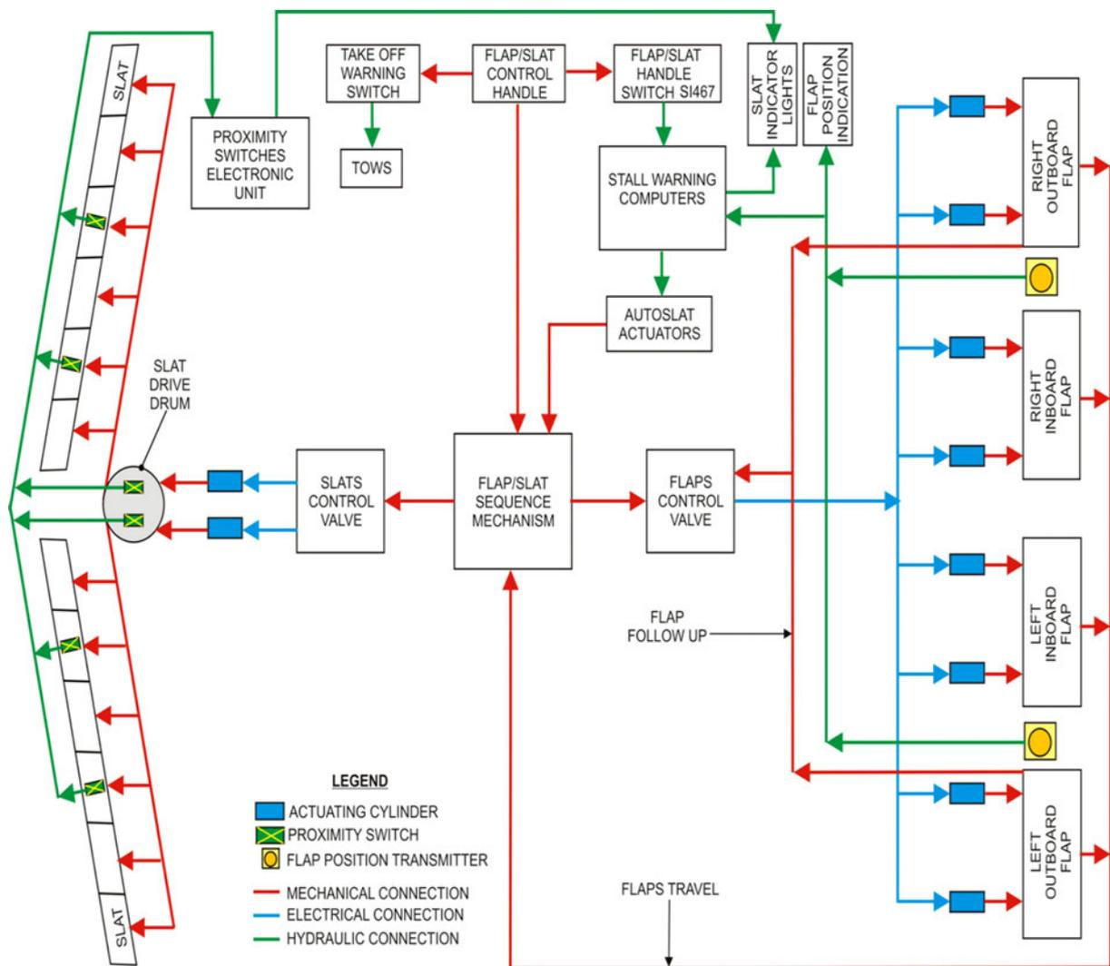
Figure 1. General diagram of flaps/slats system
