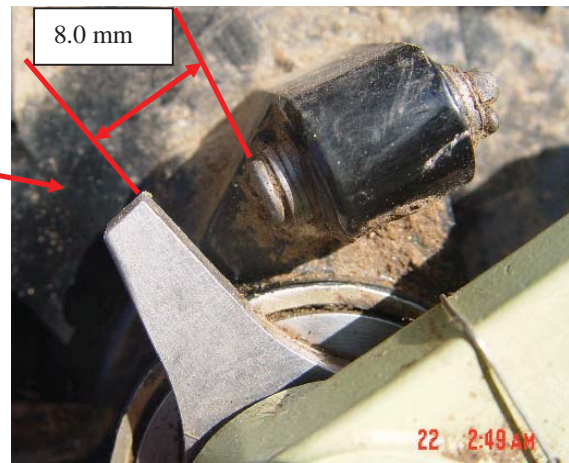
Photo - Aft Outflow Valve at accident site
