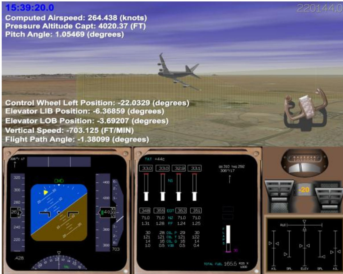
Figure 43 - GPWS: Bank Angle Warning - 15:39:19 UTC
