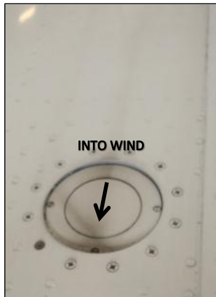
Photo 11 Smoke shutter fuselage cut-out from exemplar aircraft
