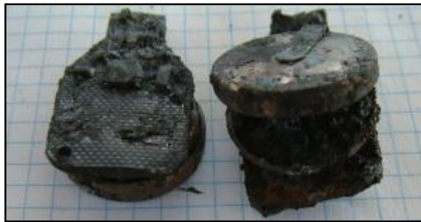
Lithium primary button sized flat cell batteries (watch style) with small circuit board
