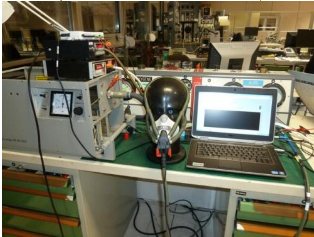
Figure 64 : Photo of MC10-25-104 comfort test set-up
