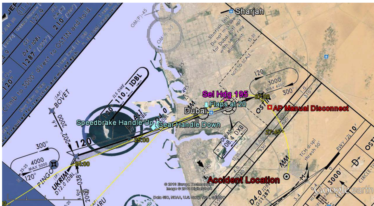
Figure 3 DXB Overview and Track [Yellow]/SHJ location and required heading for SHJ RWY 31 localizer interception
