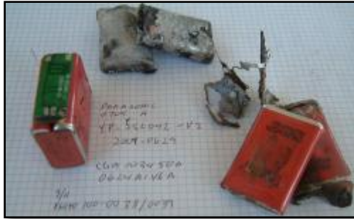
Intact and fire damaged Panasonic batteries (2-pack Li-ION set)[LH]/Mobile phones and batteries [RH]
