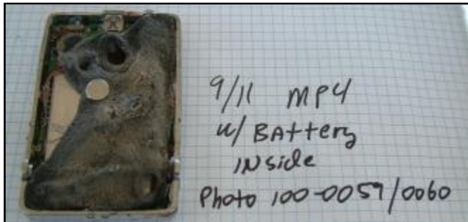
Personal electronic device with battery inside [LH]/Lithium-ion battery pack [RH]
