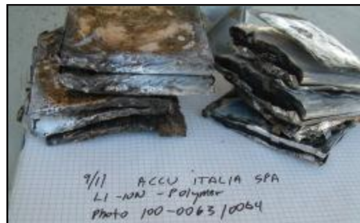
Lithium-ion polymer type battery pack [LH]/ Lithium-ion polymer type battery pack with thermal damage [RH]
