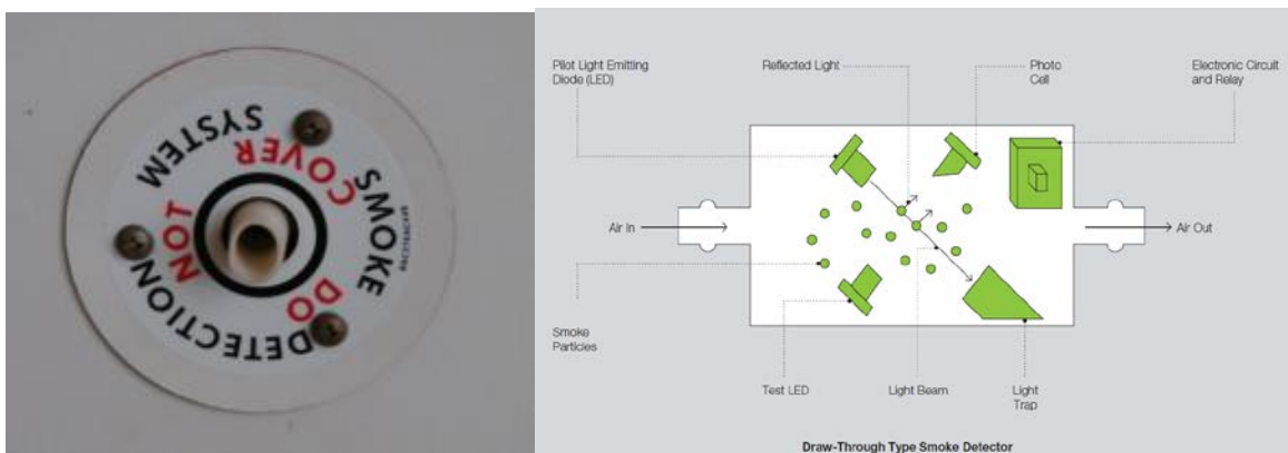
Figure 20 Draw-through Smoke Detector
