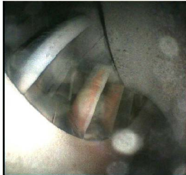
Figure 4. 1 st Stage Turbine Stator Nozzle with Acceptable Nozzle Vanes
