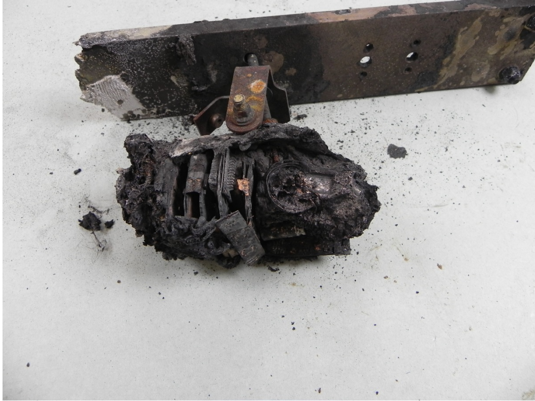
Figure 6a. Postaccident condition of onboard image recorder.
