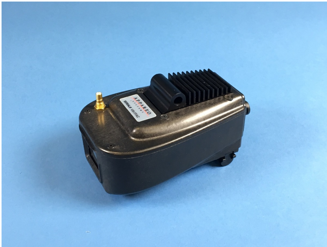
Figure 6b. Exemplar Appareo Vision 1000 onboard image recorder.
