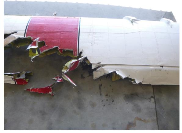
Figure 10. DHC-2 right wing with mechanical cuts that progressively penetrate inboard.
