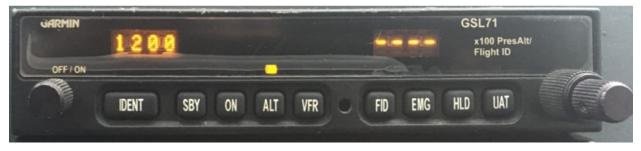
Figure 7. Photo of an exemplar GSL 71 that is transmitting pressure altitude.
