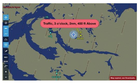
Figure 5. Example of a ForeFlight visual traffic alert with a traffic pop-up display.
