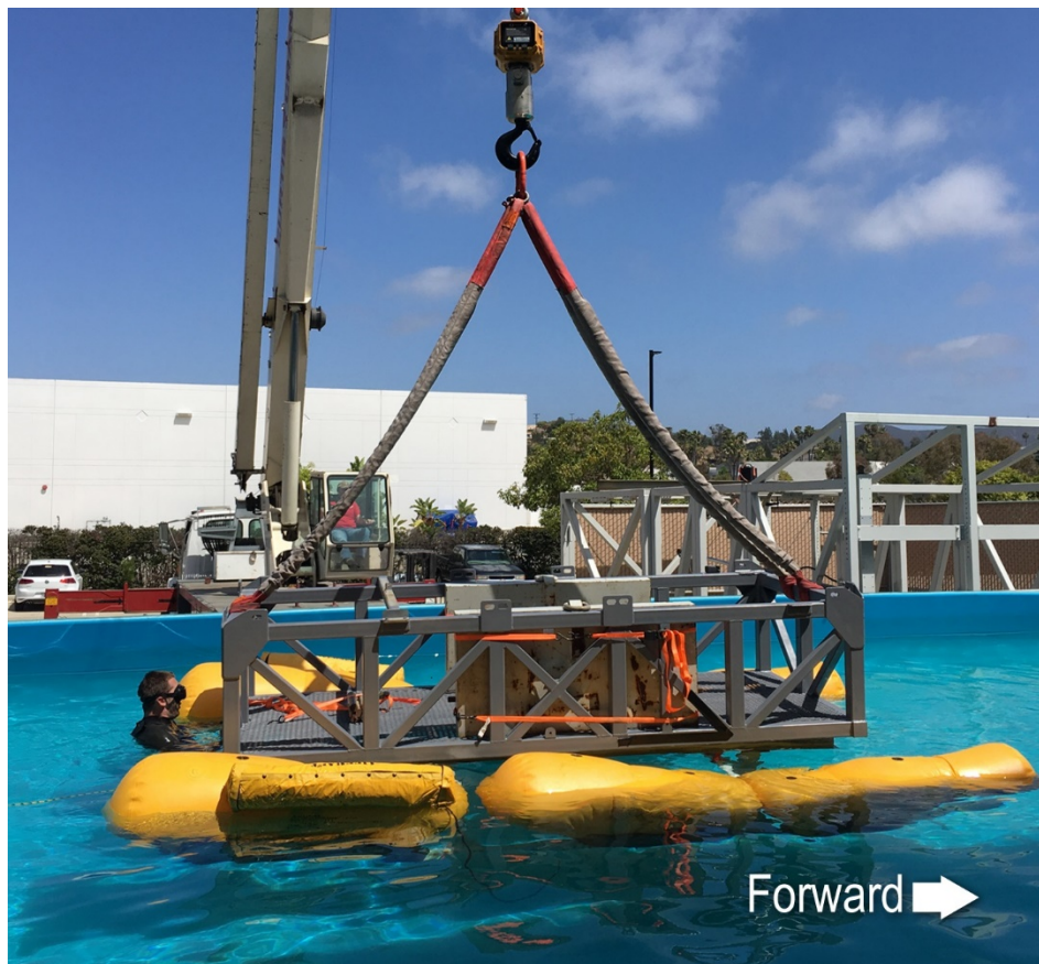
Figure 19. A test rig with partially, symmetrically inflated floats is shown suspended by a crane and lowered into a pool.
