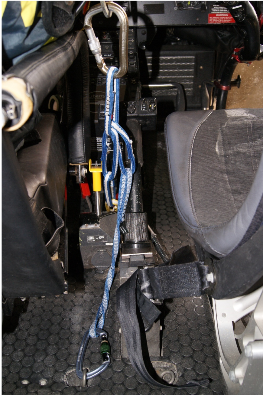
Figure 14. Front passenger's tether from the accident flight with top locking carabiner inserted through third webbing loop (from floor) with three excess loops hanging as a tail.
