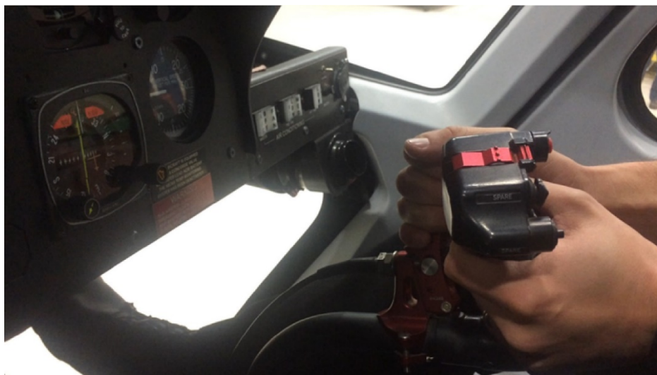
Figure 18. Screen capture from a Liberty-provided video of a test activation of the Dart emergency flotation system.
