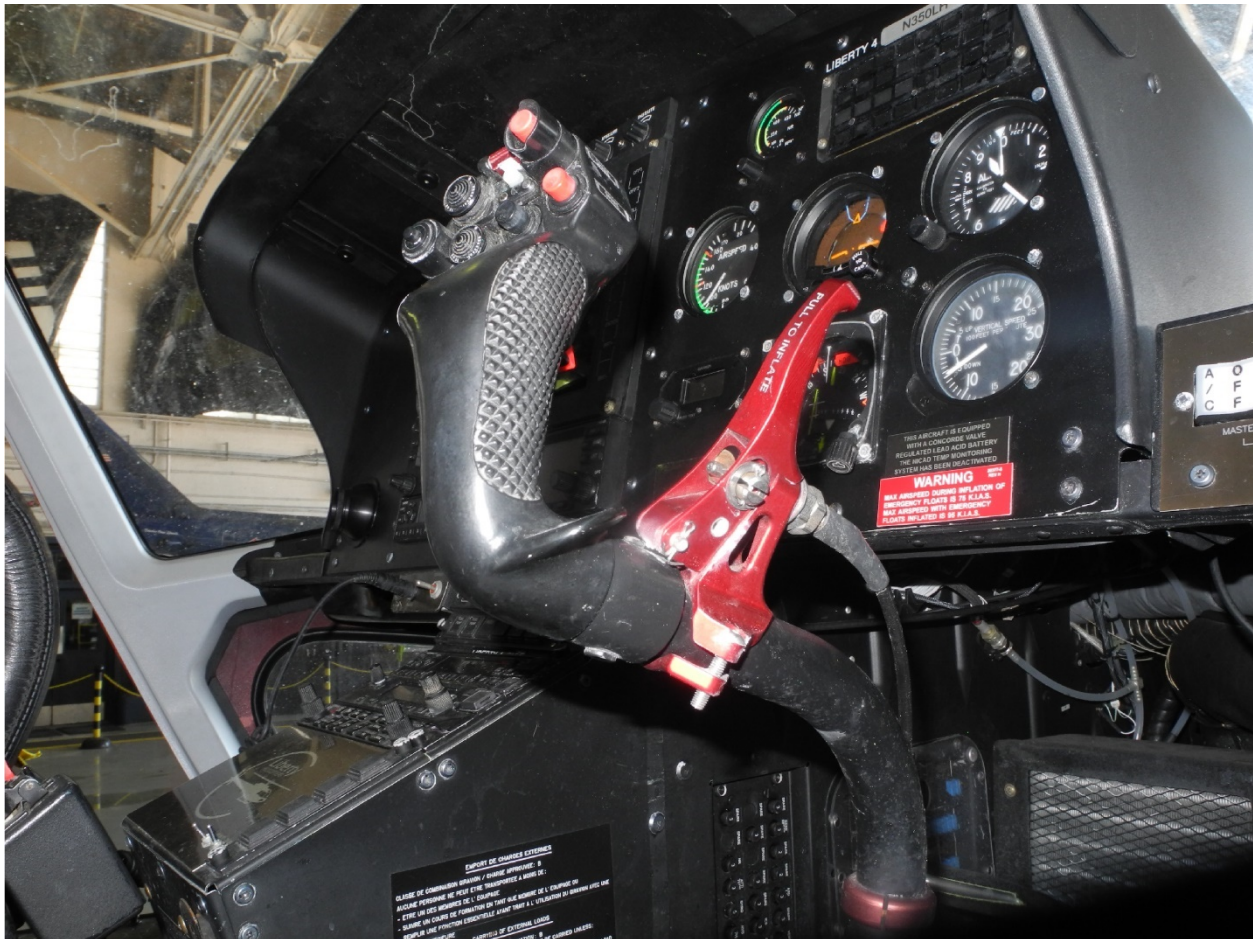
Figure 6. Float activation handle (red) installed on the accident helicopter's cyclic control.
