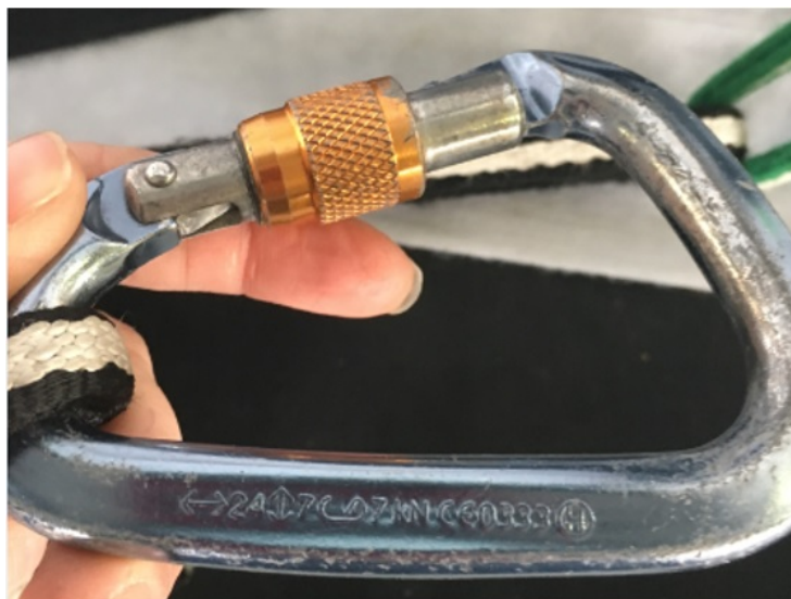
Figure 12. An exemplar locking carabiner used on a tether on the accident helicopter.
