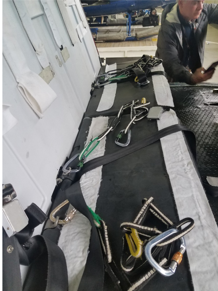
Figure 15. Rear passengers' tethers from the accident flight secured to anchor points on the aft bench bar with locking carabiners.
