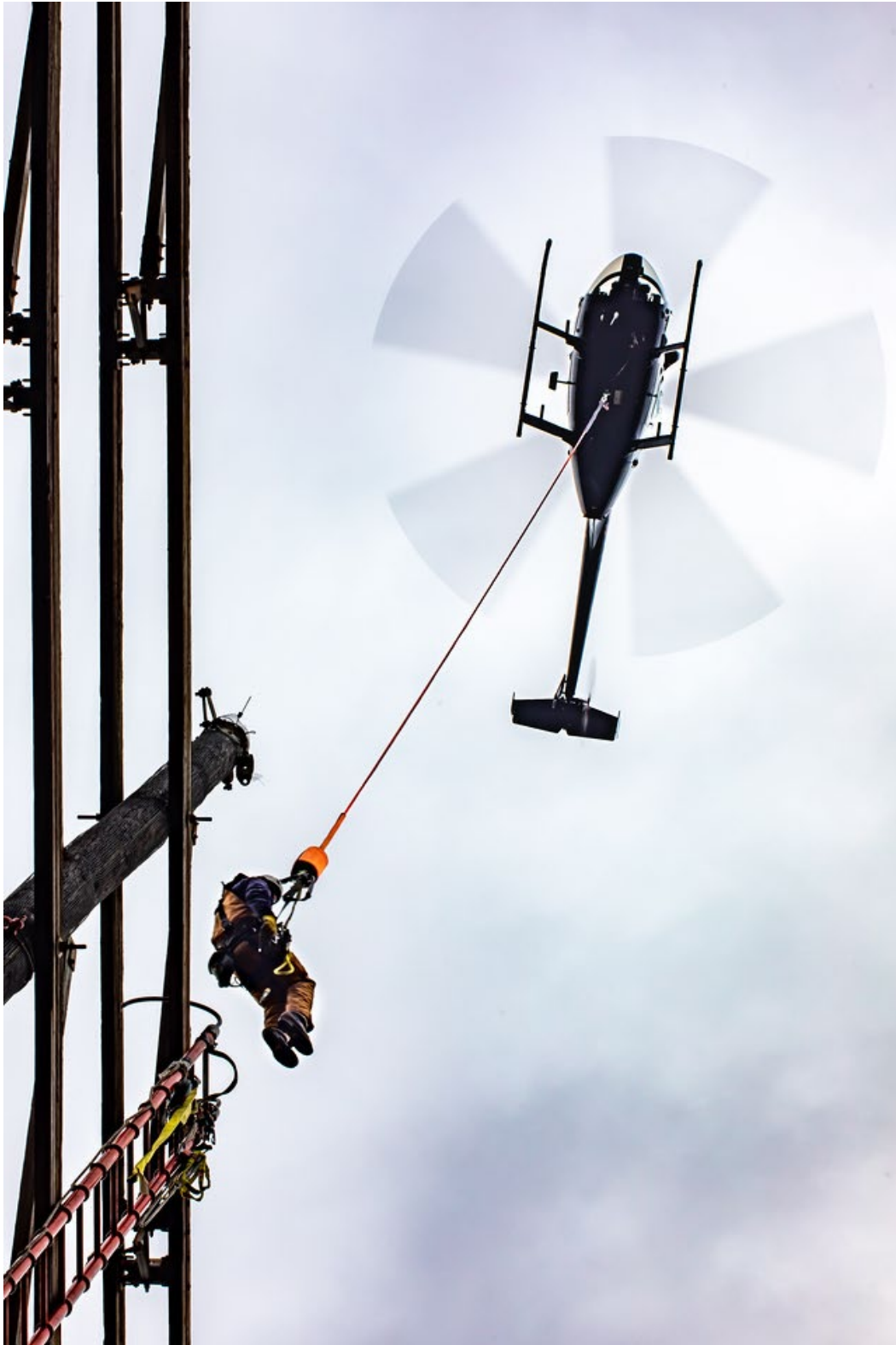
Class B HEC Operation with an FAA approved hook. Source: Mike Reyno/Brent Bundy
