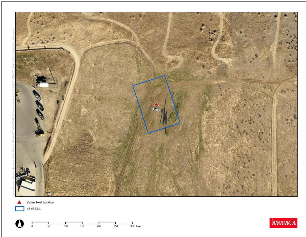
Figure 4: DNL 45 dB or Greater Noise Exposure at South Jordan/Salt Lake City Nest Location
