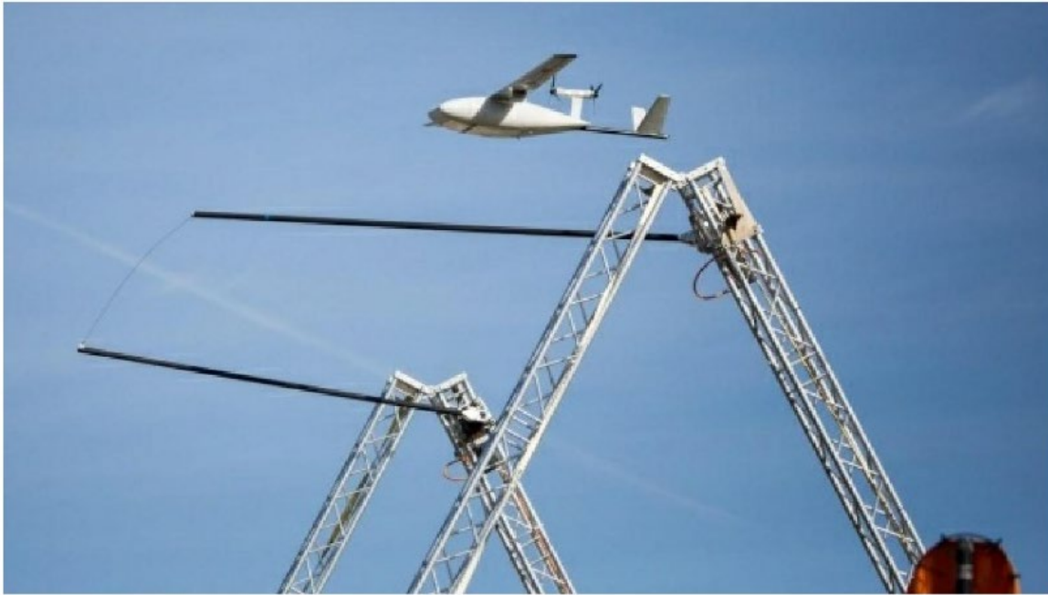
Figure 7. The Recovery System Raising to Recover a Returning UA
