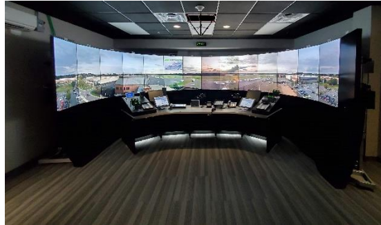
Remote Tower Module (Equipment, console, and displays)
