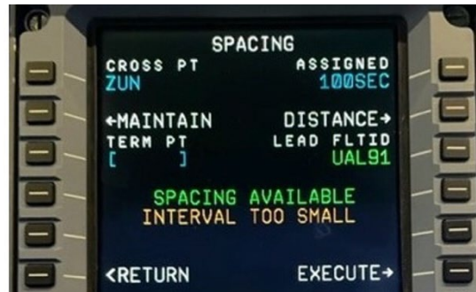
Figure 16 - SafeRoute+ Spacing application infeasibility notification on the MCDU
