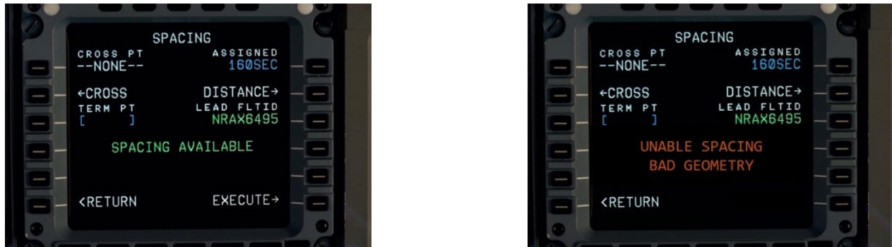
Figure 49 – Left: MCDU Spacing page for Maintain Operation; Right: MCDU Bad Geometry Message on Maintain page
