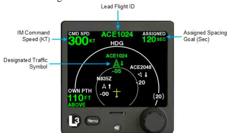
Figure 48 - ADS-B In Guidance Display as modified for the SafeRoute+ Spacing application
