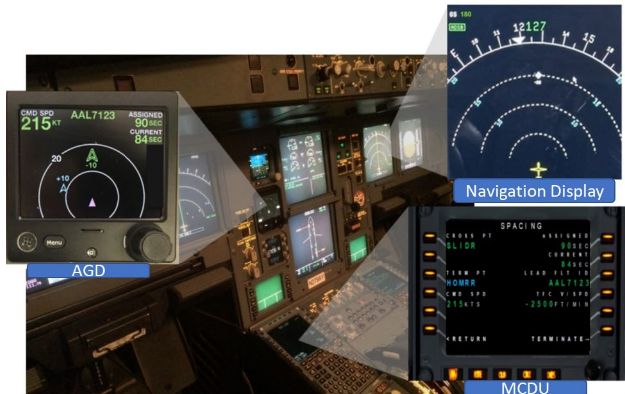
Figure 3-2. Flight Deck Avionics (clockwise from left: AGD, traffic display, and MCDU)
