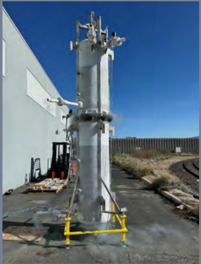
A LOX/methane test article (sized for a 2000 lb. load of propellants) undergoes tests at contractor facility. It was successfully used in the inert drop test for risk reduction after being filled with cryogenic liquid nitrogen.
