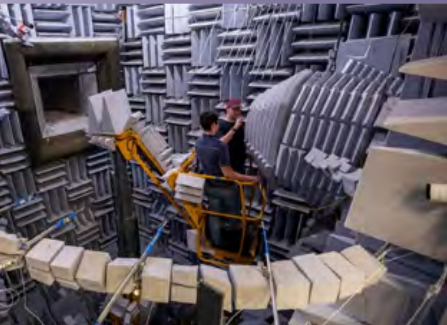
Georgia Tech graduate student Jackson Larisch and recent graduate Reagan Mayo install a test nozzle in GTRI's Anechoic Static Jet facility, where banks of microphones record sound from the nozzle as air passes through, while other instruments measure air flow velocity and pressure. (Credit: Sean McNeil, GTRI)
