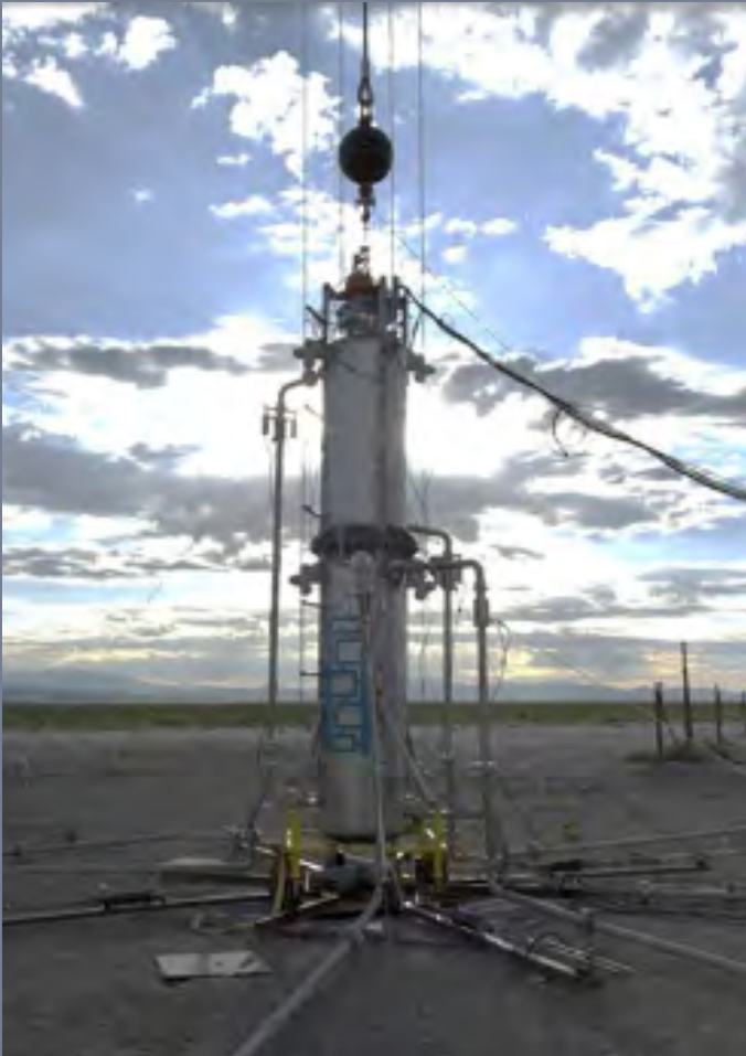
A test article is prepared with instrumentation prior to being remotely loaded with LOX and liquid methane propellants for the first explosive drop test on August 18, 2023.
