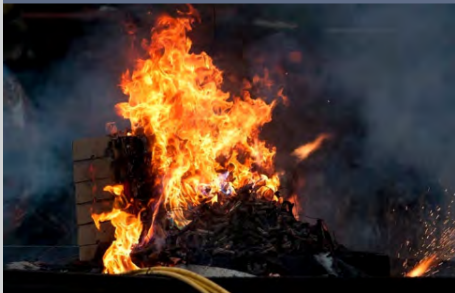
Thermal runaway consumes an entire cargo pallet of lithium batteries in minutes.
