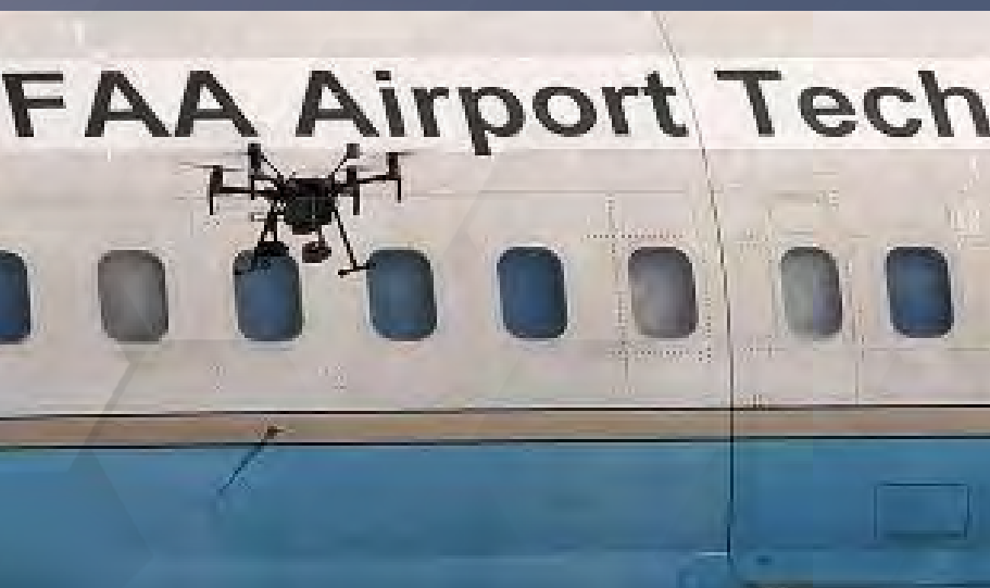
A compliant drone inspects the FAA's Boeing 727 while broadcasting remote ID messages during a demonstration of Remote ID at the William J. Hughes Technical Center.
