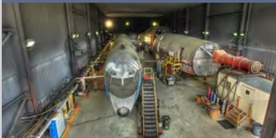
The FAA uses actual aircraft fuselages and cargo compartments to test and evaluate causes of aviation fires and the latest means of suppression and prevention.
