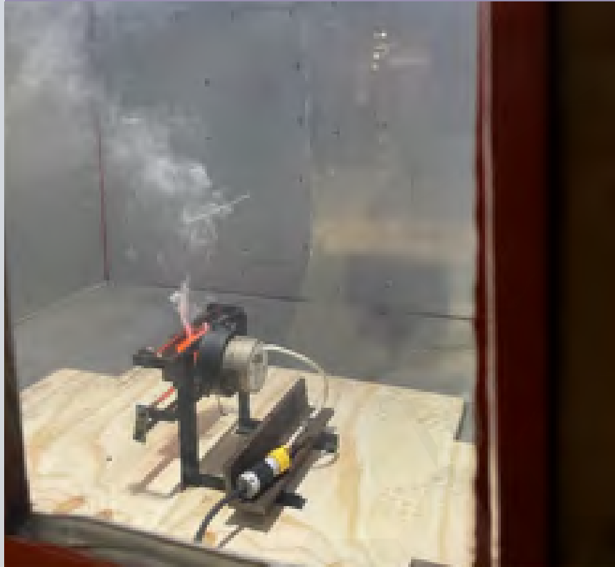
Overheating of printed circuit board substrate material.
