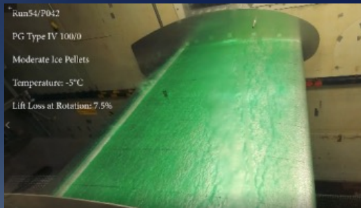
Ice Pellets with Type IV anti-icing Fluid Test (Video Screen Capture)
