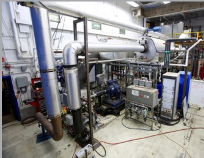
The FAA uses special equipment to research high-octane unleaded fuel replacements for current leaded aviation gasoline.
