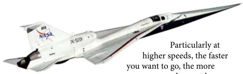
An experimental aircraft designed to test sonic boom shaping. (NASA photo by Jim Ross)
