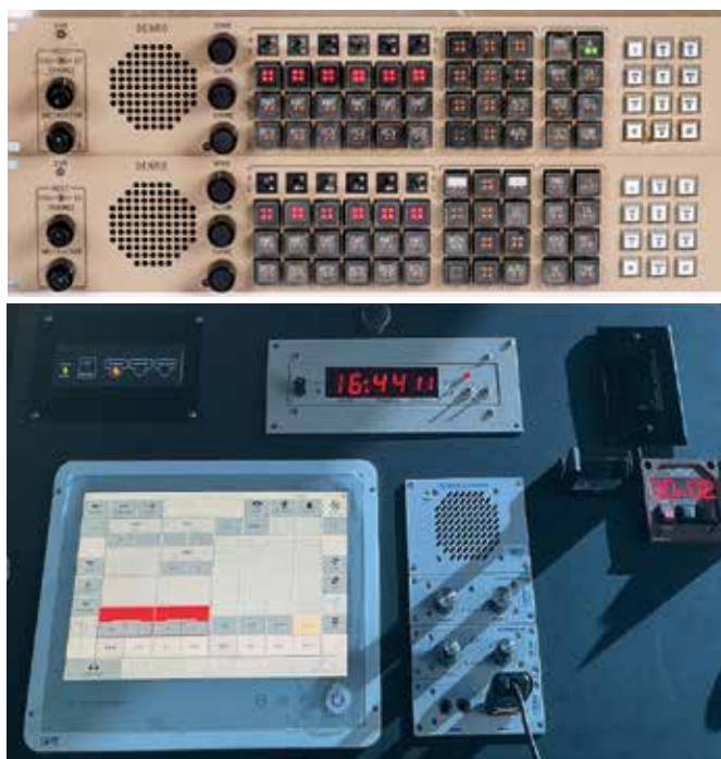
Old vs. New: The FAA is replacing analog voice switches (top) with digital (bottom). Air traffic controllers can more easily switch frequencies with greater reliability using new digital equipment.
