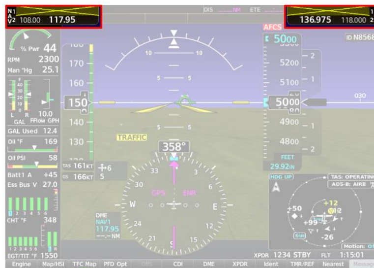
Figure 4: Single GIA Fail (Displayed in reversionary mode)
