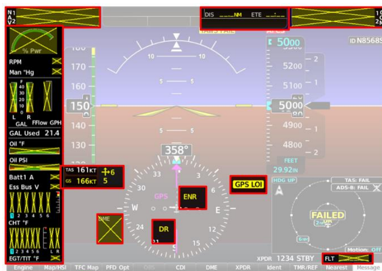
Figure 5: Dual GIA Fail (Displayed in Reversionary Mode)
