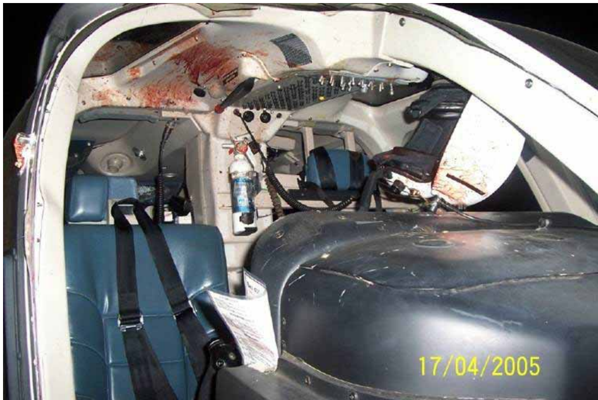
A Bell 407 air ambulance helicopter en-route at 1,000 ft AGL hit three blue-winged teal during a flight to an automobile accident in South Dakota in April 2005. The windshield shattered and glass and duck blood were splattered through the aircraft, temporarily blinding the pilot. The pilot recovered and made an emergency landing on a road.
