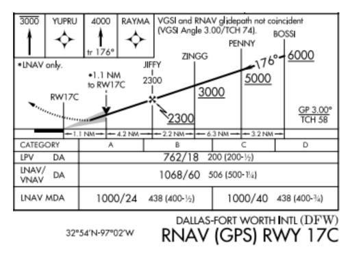
An aircraft descending using VNAV, which is generated by WAAS/SBAS and not Baro-VNAV, and on the vertical path would cross below the published altitudes at PENNY, ZINGG and JIFFY if BOSSI is designated at the FACF in nav-database coding.
