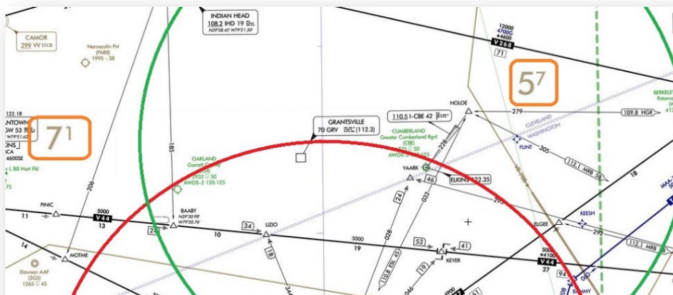
Figure 6: ESL VOR/DME Radius vs KCBE Radius on L-23
