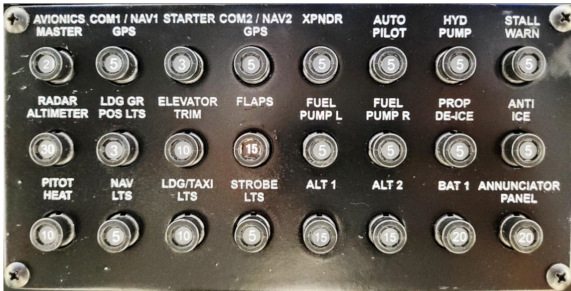
Figure 4 TAGARS Overhead Circuit Breaker Panel
