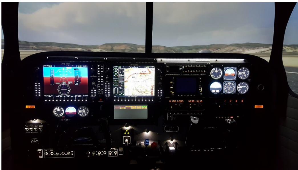
Flight Deck of the TAGARS Representing a Piper PA 46-350P (Malibu Mirage)
