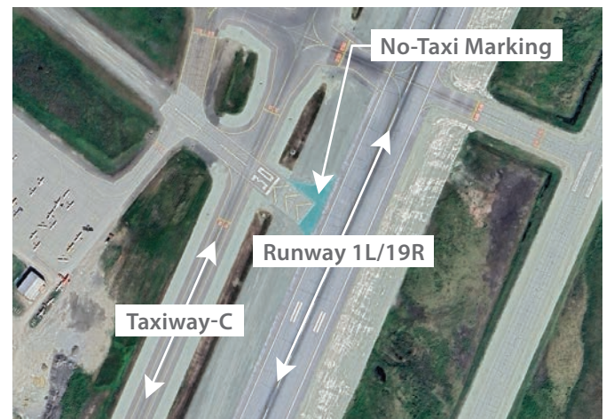
Figure 2: Aerial and side view photo (below) of a RIM project at Bethel Airport (BET) to address a confusing runway intersection.
