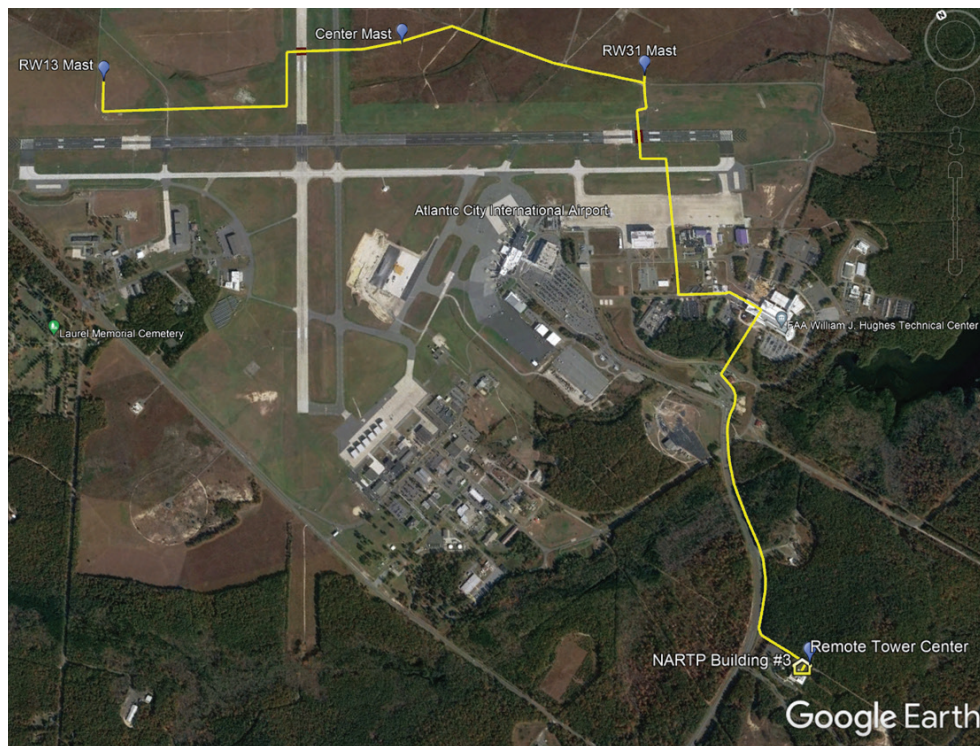
Google Earth map indicating the position of the Remote Tower System at ACY, including camera locations and Remote Tower Center.
