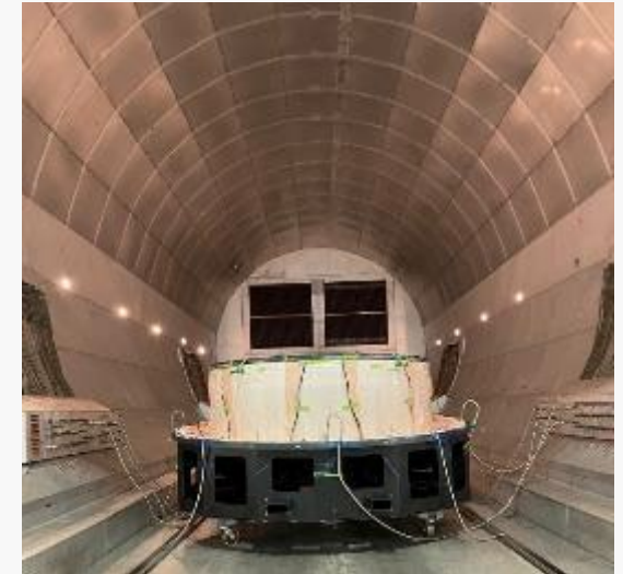
Acoustic Inner Barrel in Autoclave
