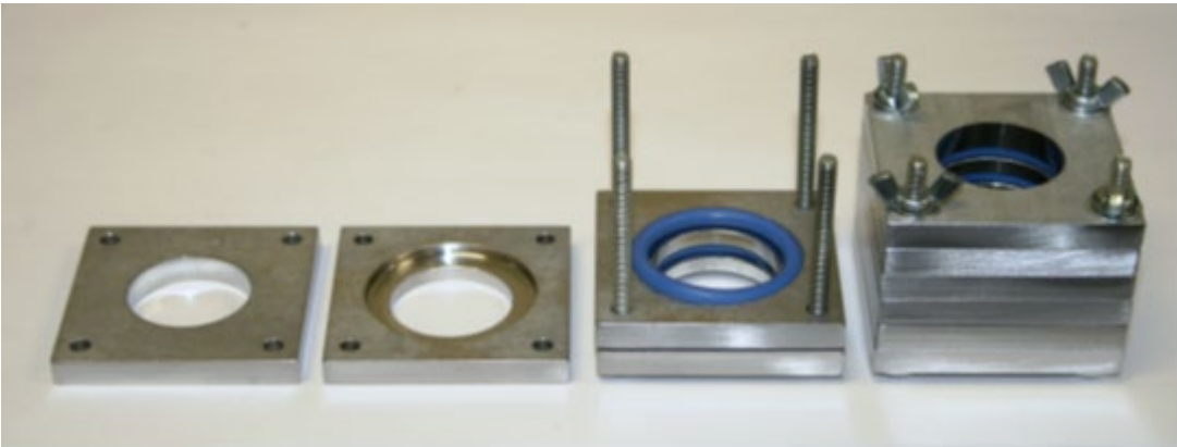
Compression set fixtures designed to constrain O-rings in a model gland to mimic the conditions of an internally pressurized seal and produce aged samples
