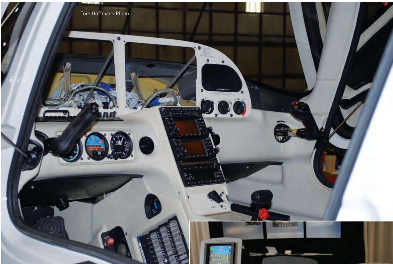
A cockpit in the midst of being upgraded to newer avionics
