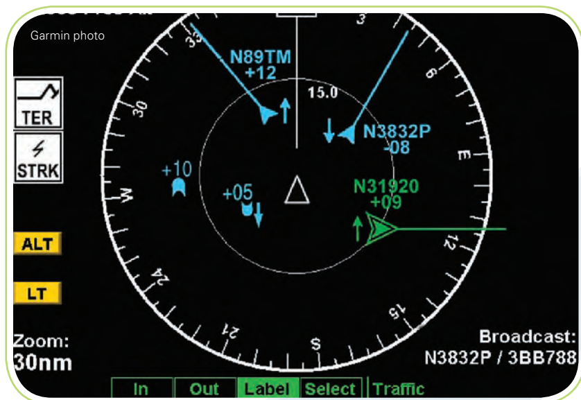
A cockpit display showing ADS-B and non-ADS-B traffic
