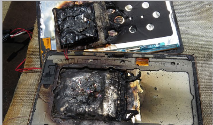
Laptop computers are among several types of personal electronic devices that can catch fire due to thermal runaway in the batteries that power the equipment.
