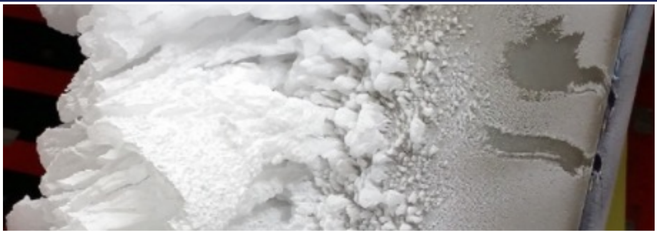
Ice builds up on a large-scale, three-dimensional swept wing during testing.
