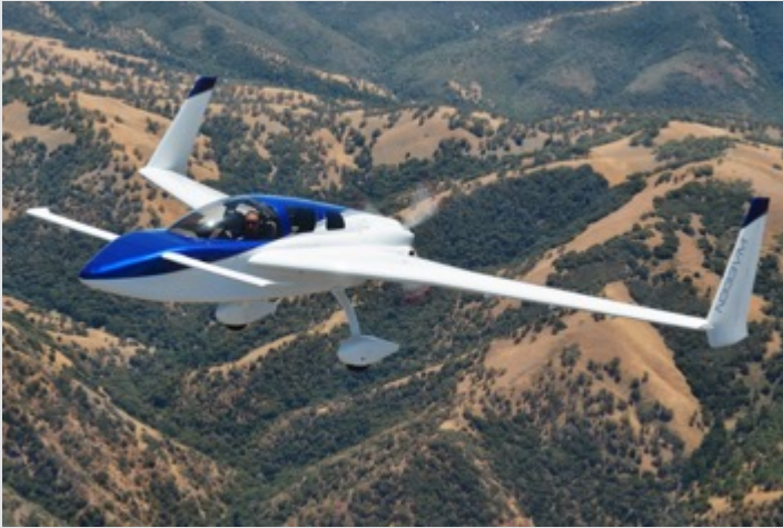
Researchers use a Cozy MK IV aircraft to test the Expandable Variable Autonomy Architecture, an enhanced autopilot technology for general aviation.
