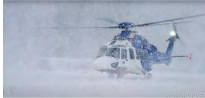
or ice can separate from the airframe inlet surface and get ingested into the engine, resulting in decreased power or engine failure.
