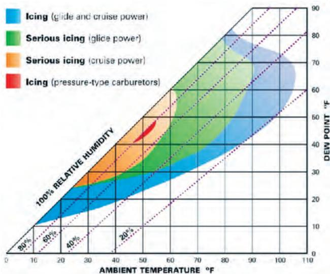
It's also worth noting that differences in engine airflow and cowling design make some aircraft types more prone to carb ice than others. For example, due to engine design and carburetor placement, a high-wing Cessna 182 with a big-bore Continental engine is more likely to build carb ice than a Lycoming-powered Piper *Cherokee*. Just remember that no carbureted engine is immune from carb icing, nor is a fuel-injected engine immune from impact icing.
