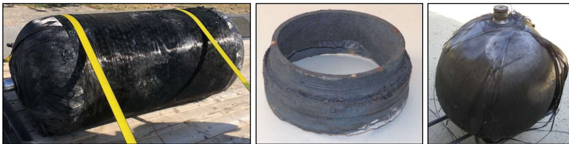
Figure 7. Photos of launch stage debris that survived reentries – Left: Composite overwrapped pressure vessel (COPV) from Falcon Stage 2 in March 2021 (Grant County Sherriff's Office, Ephrata, Washington); Center: Metal ring from engine of Falcon Stage 2 in December 2014 (The Aerospace Corporation); Right: COPV from Atlas V Centaur in March 2008 (The Aerospace Corporation).
