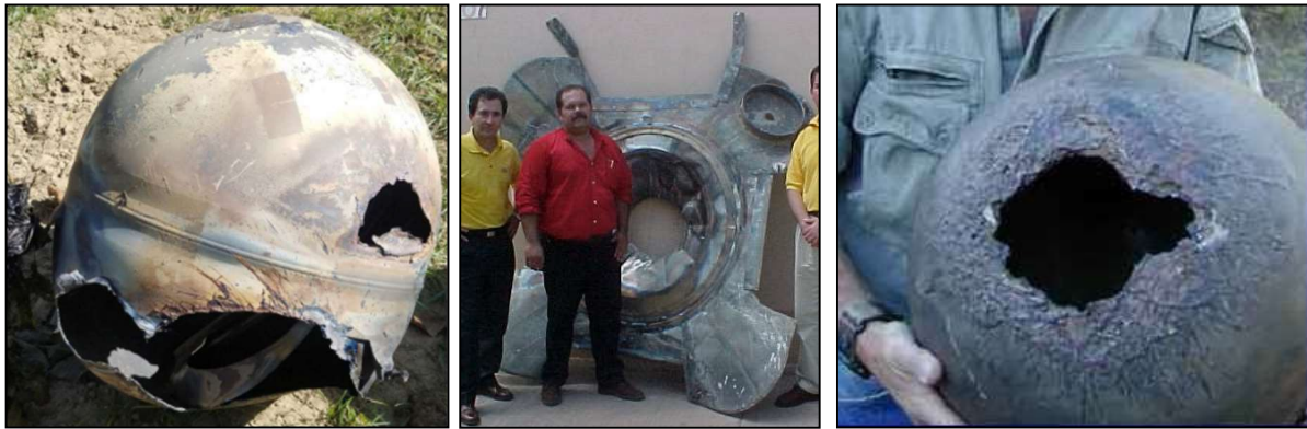
Figure 6. Photos of debris that survived satellite reentries – Left: Titanium alloy propellant tank from Iridium satellite in October 2018 (Kings County Sherriff's Office, Hanford, California). Center: Metal bulkhead from Cosmos 2267 satellite in December 1994 (Sinaloa Science Center, Culiacan Rosales, Mexico); Right: Titanium alloy propellant tank from Foton 4 satellite in April 1988 (Space.com, February 2000).
