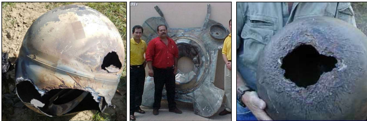
Figure 6. Photos of debris that survived satellite reentries – Left: Titanium alloy propellant tank from Iridium satellite in October 2018 (Kings County Sheriff's Office, Hanford, California). Center: Metal bulkhead from Cosmos 2267 satellite in December 1994 (Sinaloa Science Center, Culiacan Rosales, Mexico); Right: Titanium alloy propellant tank from Foton 4 satellite in April 1988 (Space.com, February 2000).
