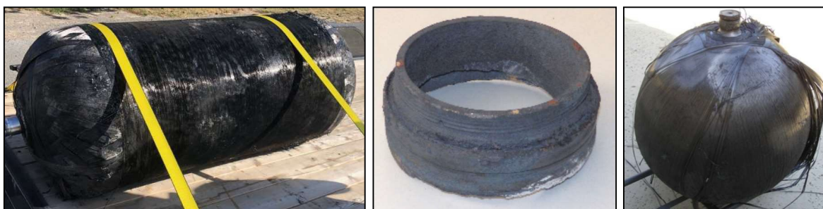
Figure 7. Photos of launch stage debris that survived reentries – Left: Composite overwrapped pressure vessel (COPV) from Falcon Stage 2 in March 2021 (Grant County Sheriff's Office, Ephrata, Washington); Center: Metal ring from engine of Falcon Stage 2 in December 2014 (The Aerospace Corporation); Right: COPV from Atlas V Centaur in March 2008 (The Aerospace Corporation).
