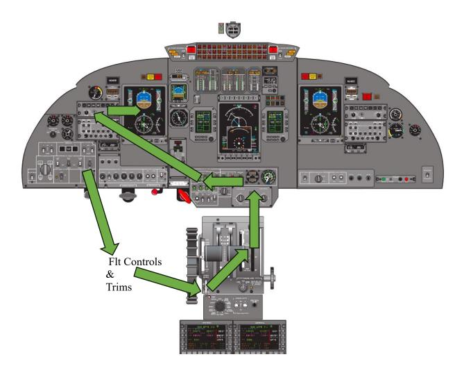
Right Pilot Before Taxi Set-up - Basic Flow Pattern (after generator checks complete)
