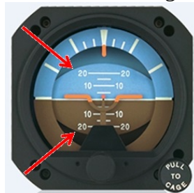
Figure 1. AIM-1200 Attitude Indicator. Note the apparent edges of the pitch indication areas of this instrument.
