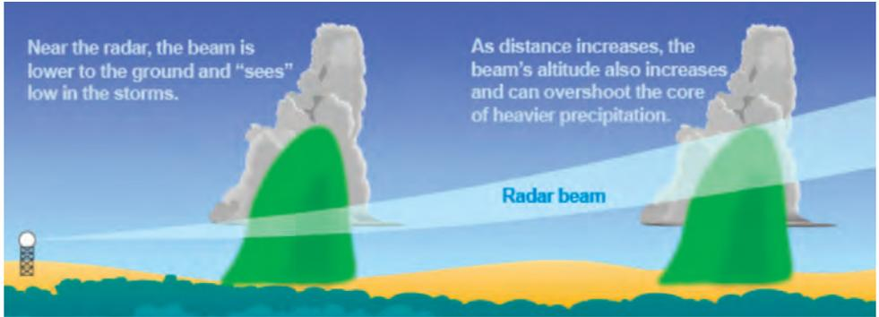
Example of a radar scanning one single elevation angle (base reflectivity).
