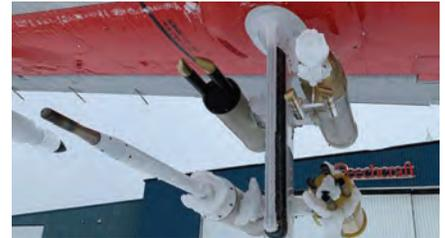
Instruments attached to the wing – including (counterclockwise from upper left) a forward scattering spectrometer probe, Rosemount air data probe, and cloud droplet probes – measure different cloud particle sizes and concentrations.
