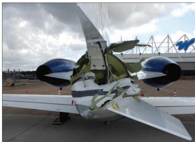
Figure 1: Aft view of tail cone damage to the Cessna Citation cited in the accident at Hobby Airport. Photo courtesy of NTSB.
