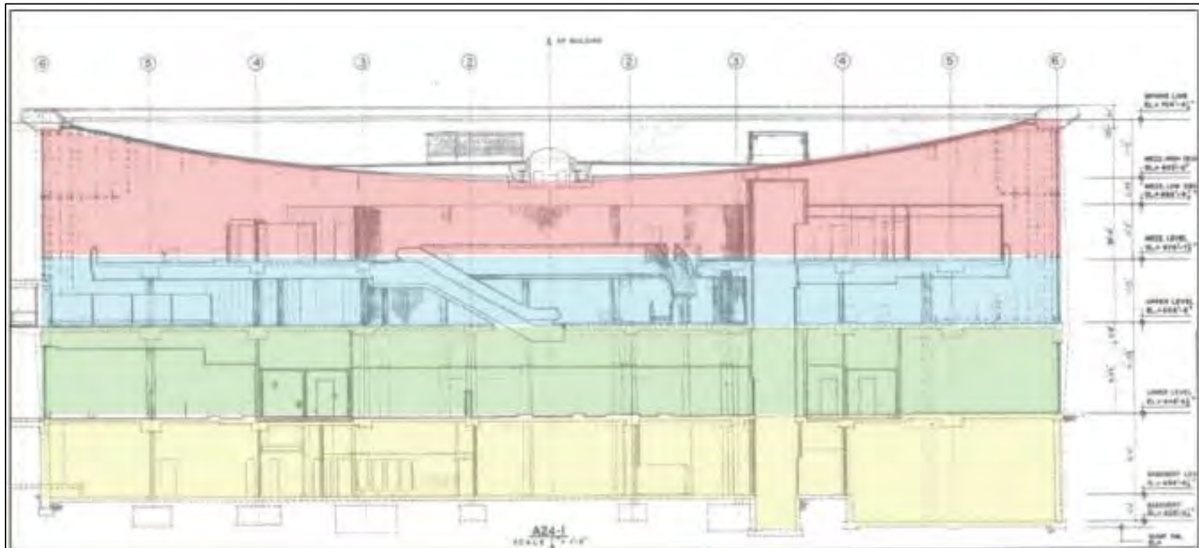
Figure 9. Excerpt from a 1964 as-built plan set illustrating the basement (in yellow), apron level (in green), concourse level (in blue), and mezzanine level (in red) within the Rotunda. Shown at center are the original escalator and concrete stairs. 7
