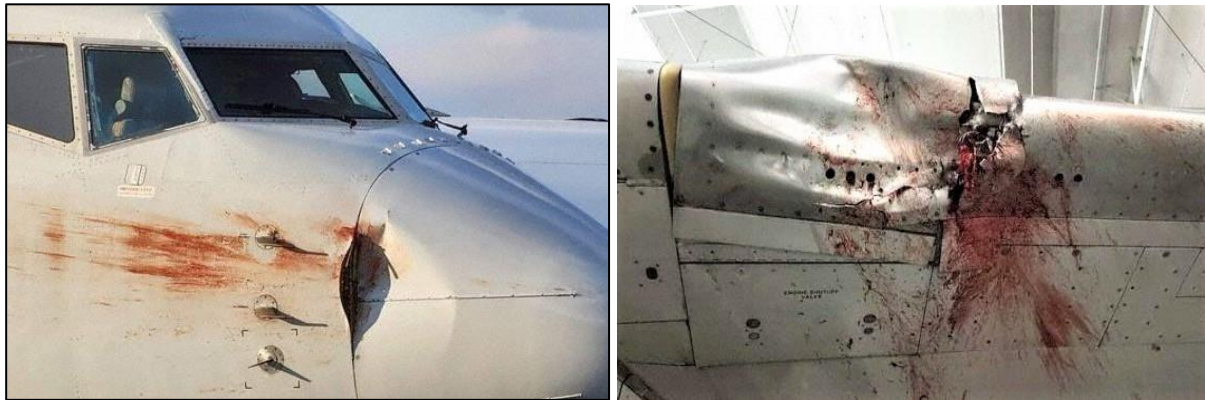
A B-737-800 on approach at night to a Midwest airport at 5000 feet AGL and 250 knots in November 2022 struck multiple Canada geese, causing damage to the radome, both wings, engine cowling, and Pitot tubes (airspeed indicators). The flight crew declared an emergency and landed safely with a visual approach 8 minutes after the strike. Photo, Roger Skorepa.
