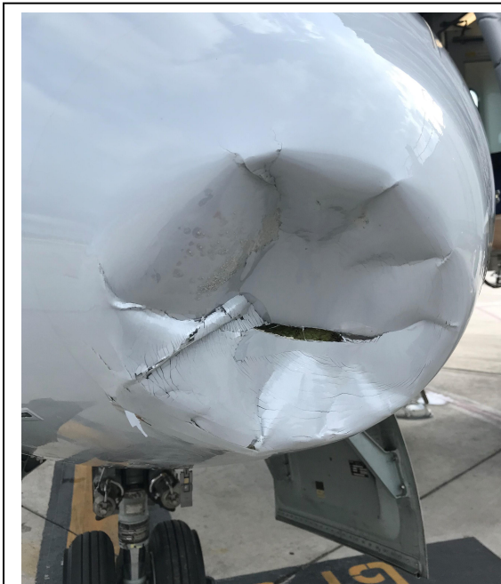
A CRJ900 struck a red-tailed hawk on departure from a Midwest airport, November 2022. The aircraft continued to its destination where the radome was replaced. In 2022, 235 red-tailed hawk strikes with civil aircraft were reported. Photo C. Mealman, USDA.
