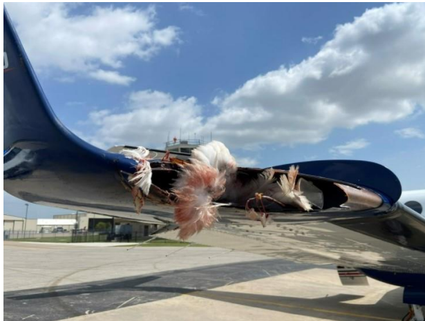
A BE-200 was on initial approach to an airport in Texas at 4500 feet AGL and 248 knots in April 2022 when an American white pelican was struck. The pilot landed the aircraft safely despite substantial damage to the right wing. The AWPE population in North America has increased 4-fold from 1990-2021 (Dolbeer 2020, Sauer et al. 2022). Photo, D. Warschun.
