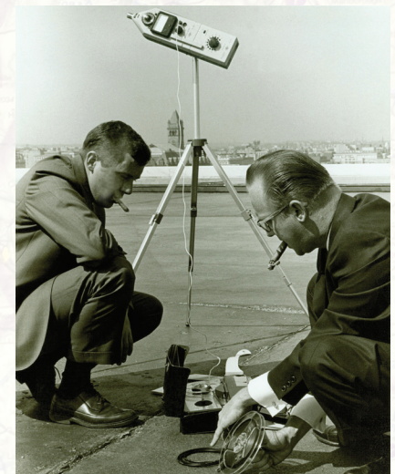
1966, FAA researchers take noise measurements on top of FAA headquarters building, Washington, DC
