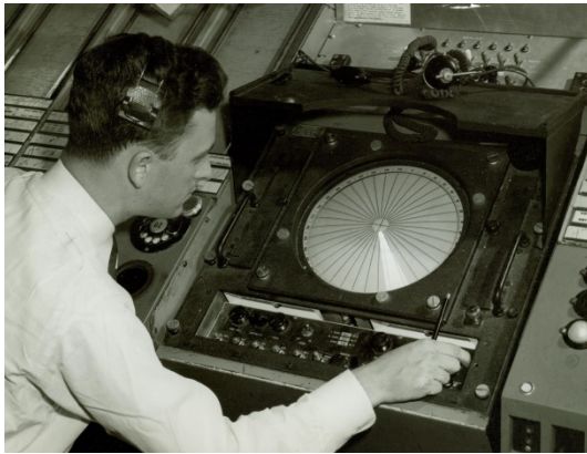
Early radar display being tested at the Washington air route traffic control center in 1948
