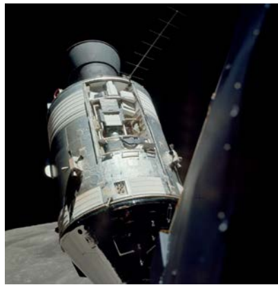
Apollo 17 SIM bay on the service module, seen from the Lunar Model in orbit around the moon
