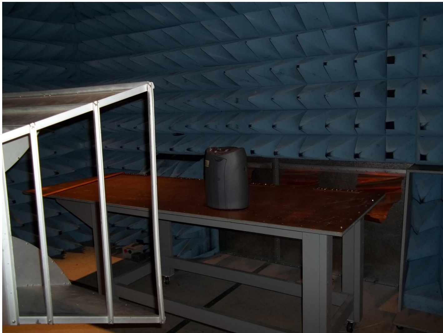
Photograph 2: SECTION 21 RADIATED RF EMISSIONS 200 MHz to 1 GHz, Double Ridge Guide 1m Setup
