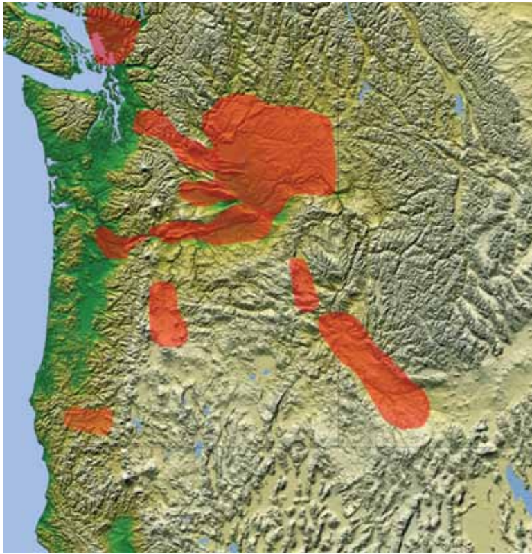
Fig. 2 – Favored locations for freezing rain in Seattle Center's airspace.
