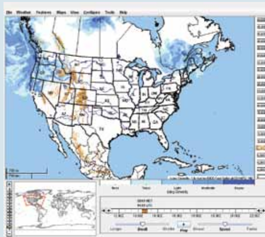
CIP depiction of icing conditions at 8,000 ft MSL from the Aviation Data Display System (ADDS) Flight Path Tool. Severity is depicted with varying shades of blue.
