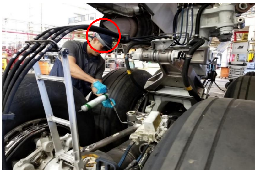
1. Image of AMT using AR to perform landing gear lubrication task (image was taken and provided by the author of this article)
