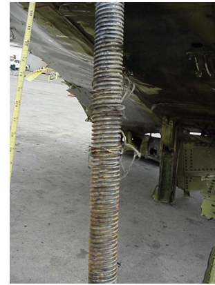
Figure 2. Jackscrew assembly recovered from Alaska Airlines flight 261 crash. Image courtesy NTSB.
