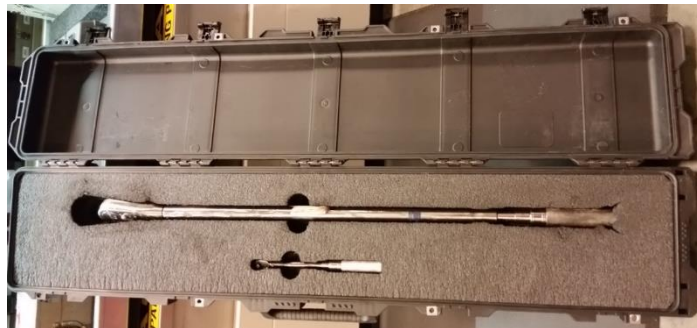
737 tire change kit designed to keep required tools together. Property of United Airlines.
