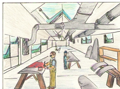
Figure 4. Doping process in a factory with ventilation, separated work process, and workers using protective aprons and goggles (based on 1918 Buffalo, NY, photo 86-5702, National Air and Space Museum) (used with permission of author)
