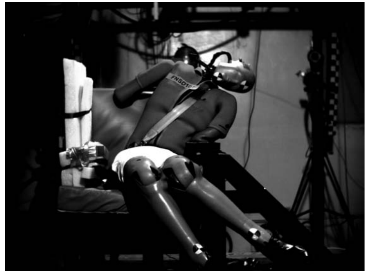
This image illustrates testing to establish neck injury criteria for side-facing aircraft seats.
