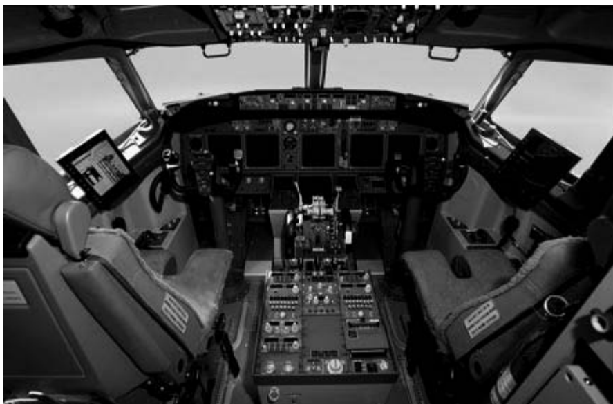
The Electronic Flight Bag (EFB) helps pilots perform flight-management tasks.
