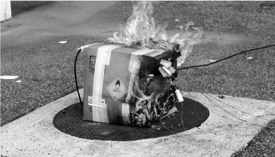
The oxygen generator over pack failed to contain a lithium metal battery fire.
