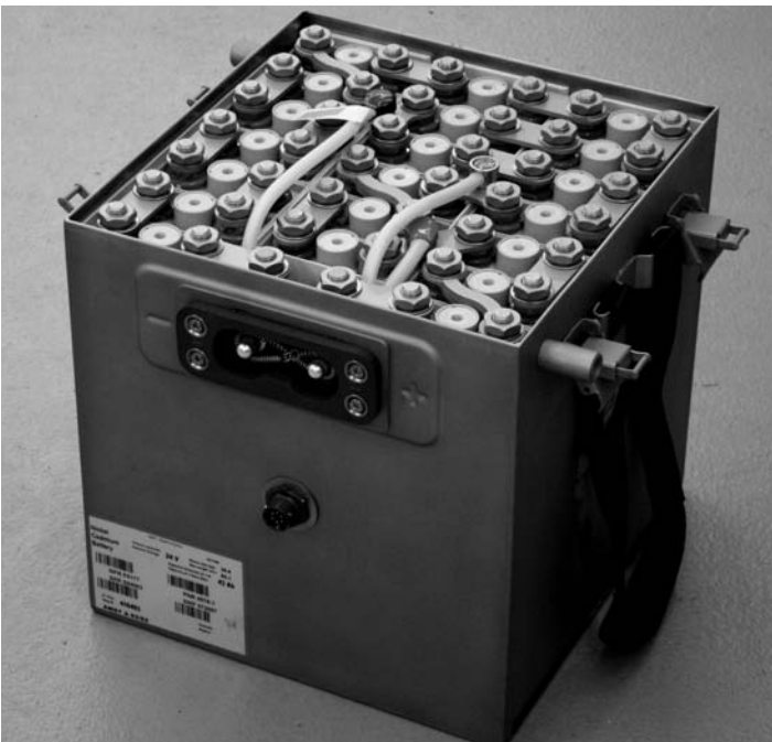
Researchers used this SAFT 4078-7 NiCd Battery in testing.
