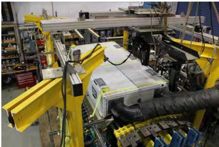
Figure 29: Test step-up used in FASTER Lab: (a) B/Ep and aluminum bonded repair patches; and (b) Environmental chamber to control temperature and humidity
