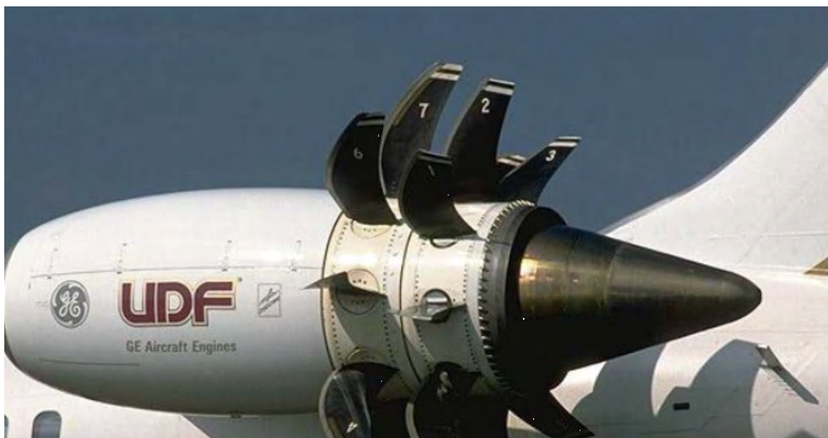
Figure 22: 1980's Un-Ducted Fan demonstrator Engine
