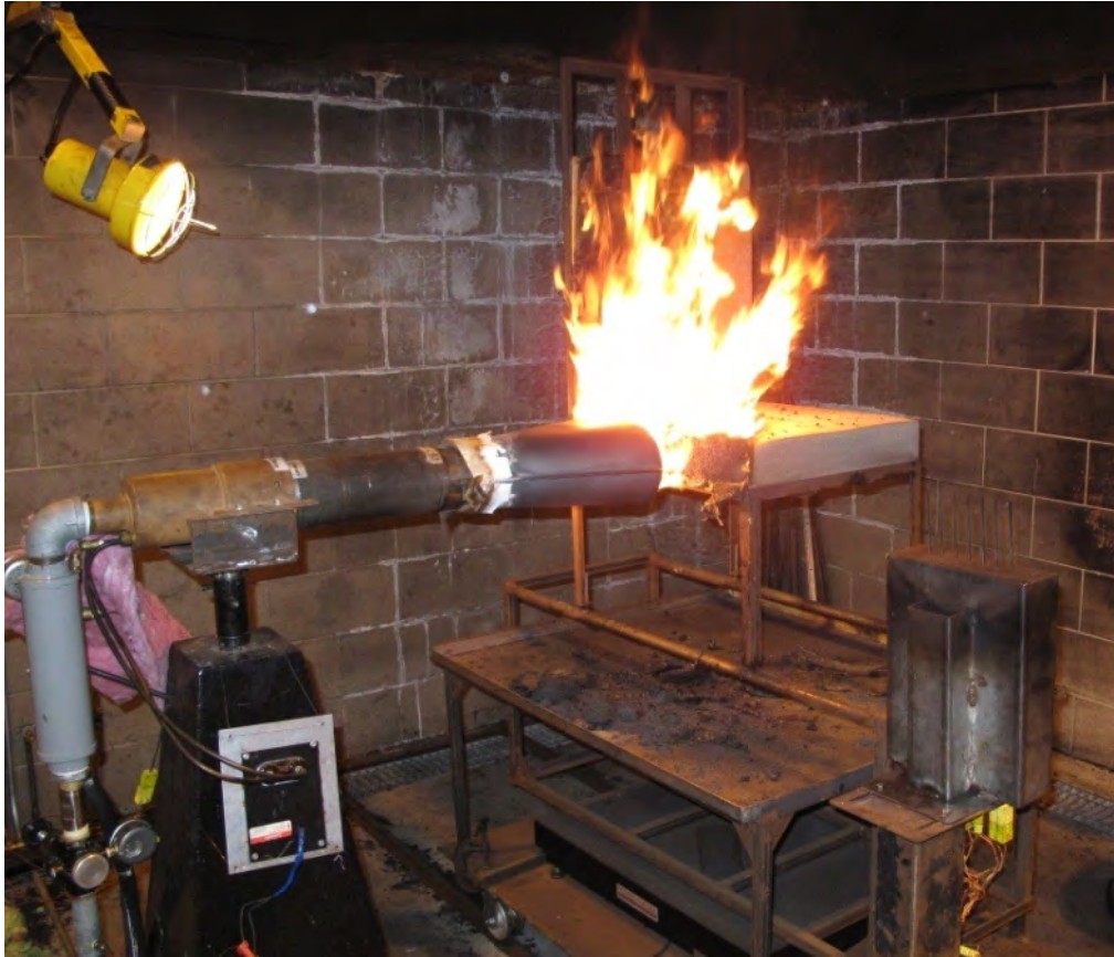
Figure 40: Aircraft seat cushion flammability test
