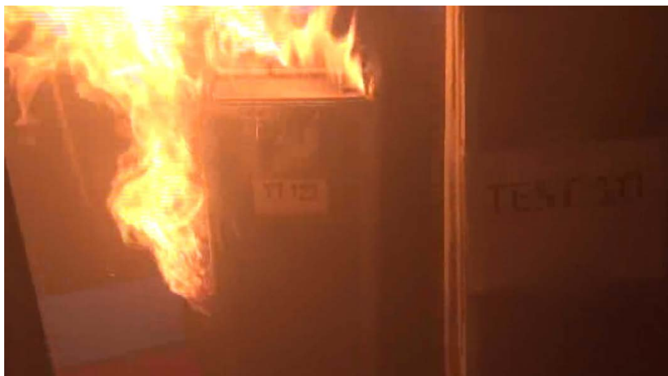
Figure 37: Flames emitted from e-tablets within a closed galley cart
