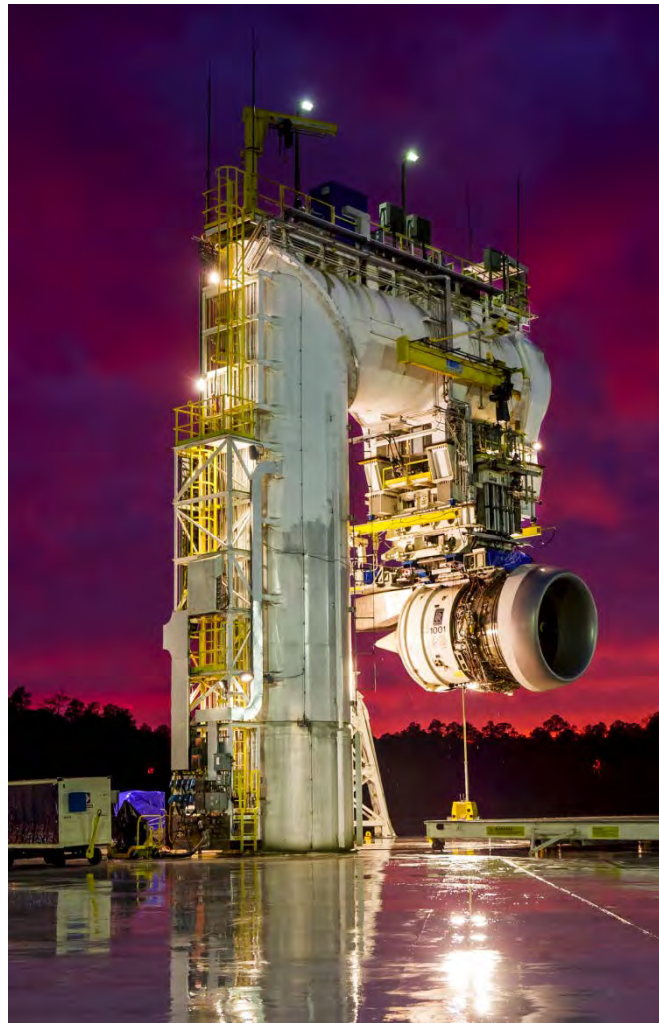
Figure 58: Boeing's ceramic matrix composite nozzle installed on a ground engine test stand
