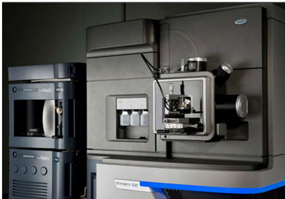
Figure 17: A Comprehensive Forensic Drug Screening Methodology was developed in the ultra-performance liquid chromatography time-of-flight mass spectrometry (UPLC-MS TOF)
