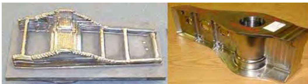
Figure 35: Aircraft parts made from additive direct energy deposition
