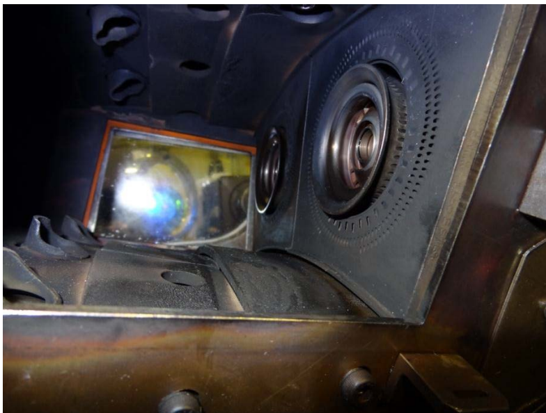
Figure 128: View Inside a Rolls-Royce Combustor that is used to Conduct Operability Testing on Candidate Fuels
