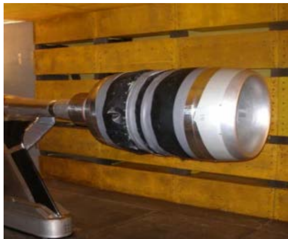
Figure 127: Pratt & Whitney's Fan Rig Model Installed in the NASA Glenn 9' x 15' Wind Tunnel
