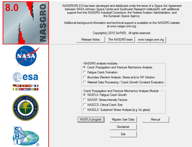
Figure 62: NASGRO ® -NASA-Developed Software Package Capable of Performing State-of-the-Art Fracture and Fatigue Crack Growth Analysis
