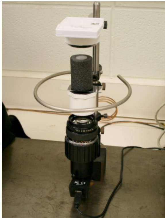
Figure 2-2. An early example of an optical dilatometer.
