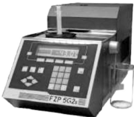
Figure 8: Automatic Freezing Point Apparatus for test method ASTM D-7153 (Source: www.astm.org )
