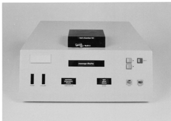
Figure 7: Apparatus Exterior from ASTM D5972 (Source: www.astm.org )
