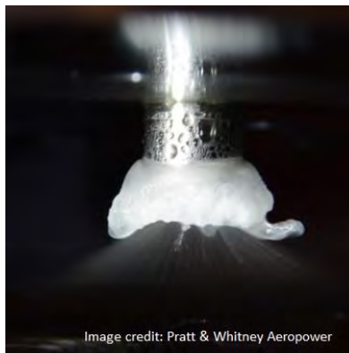
Figure 8-12. Ice Built Up Near Injector Tip
