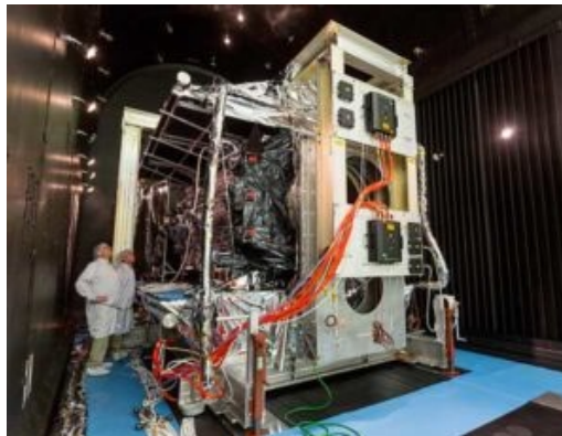
Thermal Vacuum testing verifies that a satellite can operate in space's extreme environment. (Photo: Lockheed Martin)
