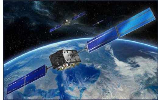
Europe's Galileo navigation satellites orbit 23,222 km above Earth to provide positioning, navigation and timing information all across the globe.
